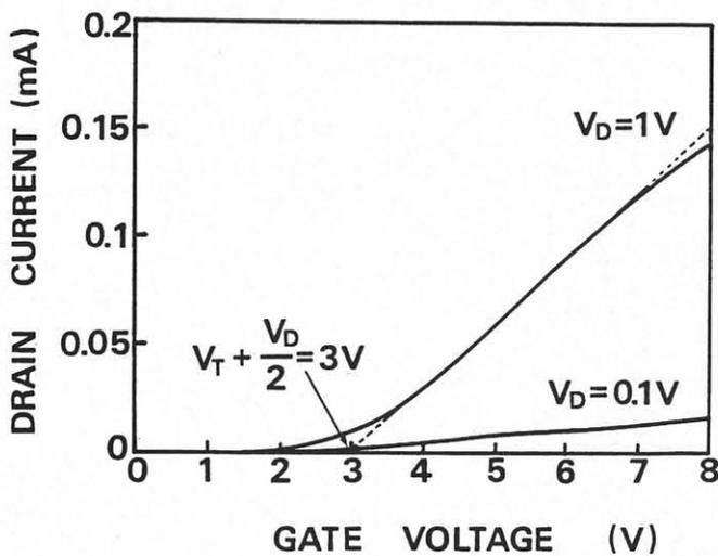
Fig.4  $I_D$ - $V_G$  characteristics of the MOSFET.
