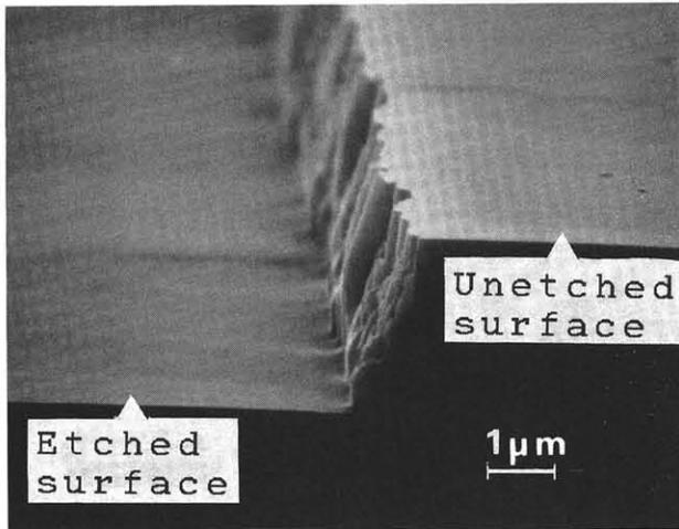
Fig.1 SEM micrograph of the  $\beta$ -SiC layer after RIE.
