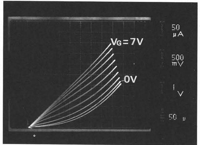
Fig.5  $I_D$ - $V_D$  characteristics of a MOSFET at 350°C.
