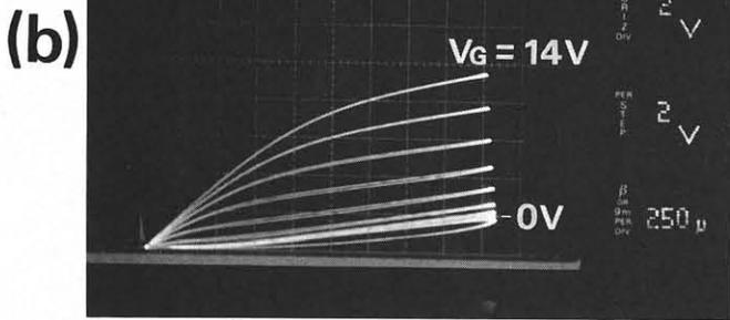
Fig.3  $I_D$ - $V_D$  characteristics of a MOSFET. (a) Drain voltage; 0-5V, (b) Drain voltage; 0-19V.
