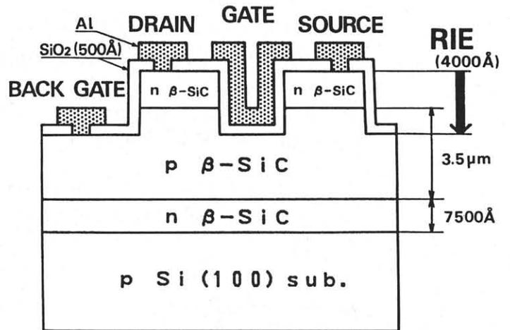
Fig.2 Schematic cross sectional structure of a  $\beta$ -SiC MOSFET.
