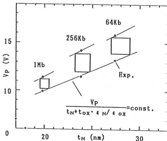
Fig. 5 Programming voltage  $V_p$  versus  $\text{Si}_3\text{N}_4$  thickness for each density of EEPROM. Upper limit of  $V_p$  varies with tunnel oxide thickness.
