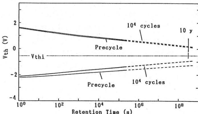
Fig. 6 Long term retentivity of MNOS memory device for 1M bit EEPROM at 85 °C.
