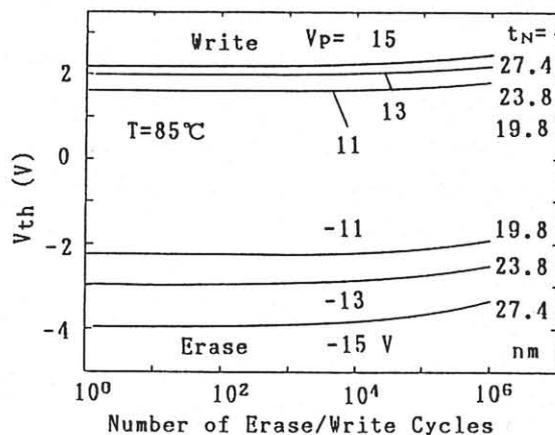
Fig. 3 Memory window versus erase/write cycles.
