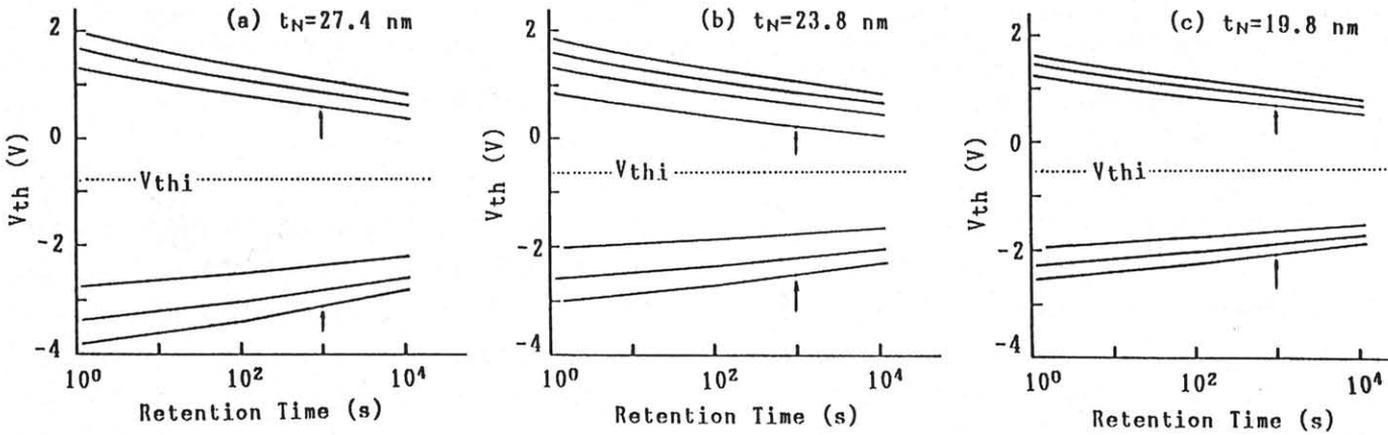
Fig. 1 Retention characteristics with various programmed threshold voltages at 85 °C.
