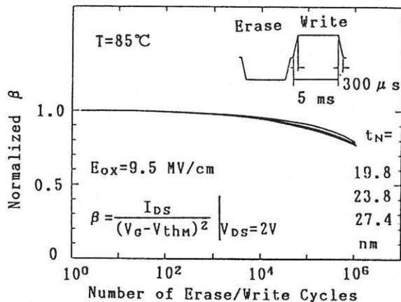
Fig. 4 Normalized transconductance coefficient versus erase/write cycles.
