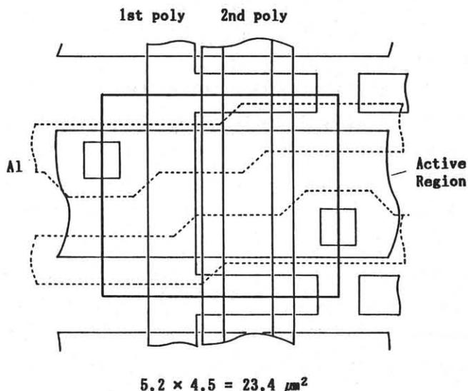
Fig. 7 Memory cell layout pattern with 0.8  $\mu\text{m}$  design rules.
