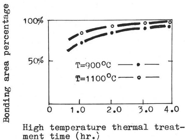
Fig.2 The relation between bonding area and high temperature thermal treatment time.
