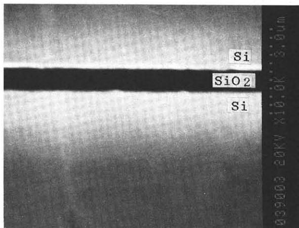
Fig.4 SEM microphotograph of the produced silicon on silicon dioxide substrate.
