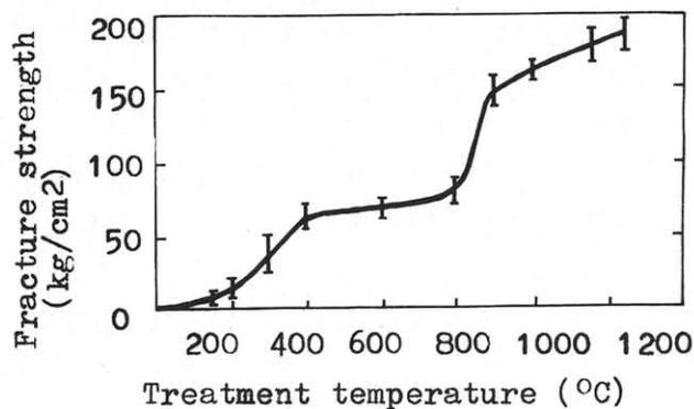
Fig.1 The relation between fracture strength and treatment temperature.
