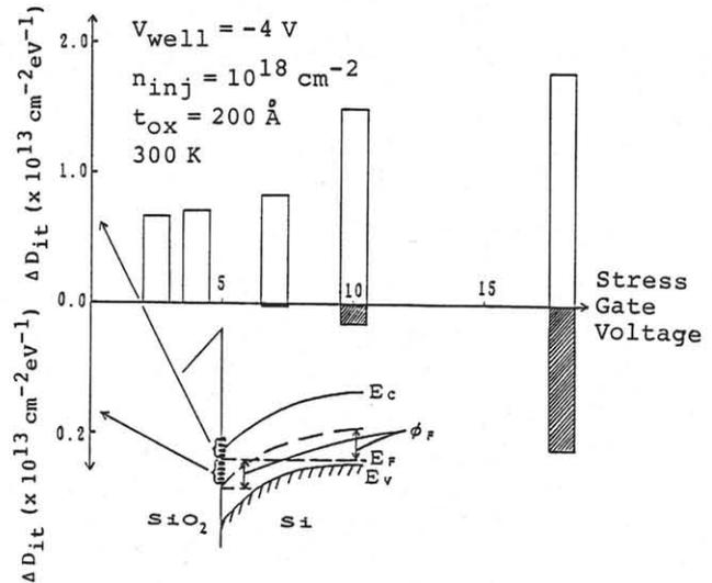
Fig. 3. Interface state density as a function of stress gate voltage. The p-well voltage was -4.0 V, and the injected electron density through the gate oxide was  $10^{18} \text{ cm}^{-2}$ .
