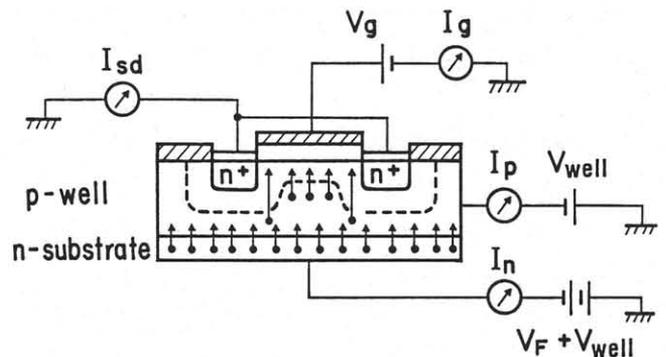
Fig. 1. Measurement circuit configuration for SHE injection.
