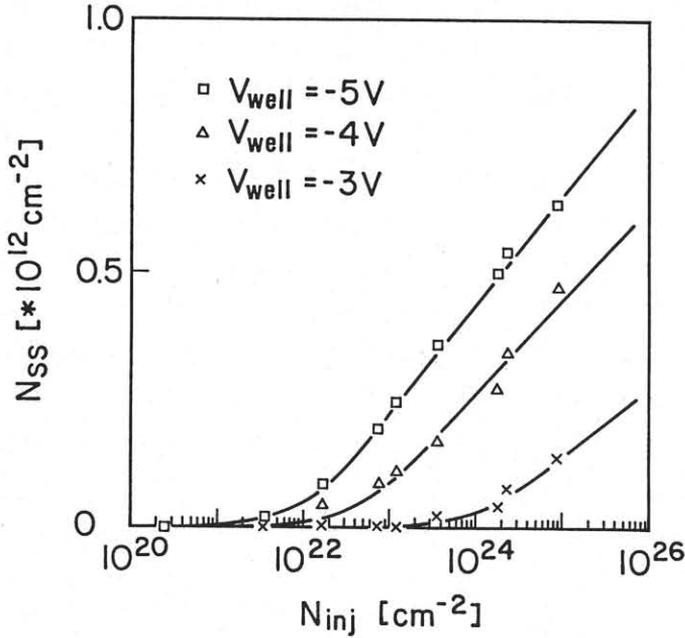
Fig. 6. Generated interface state density as a function of the electron density to the Si-SiO<sub>2</sub> interface. Squares, triangles and crosses are experimental results at stress gate voltage of 2.5 V, while the solid curves are calculated results.
