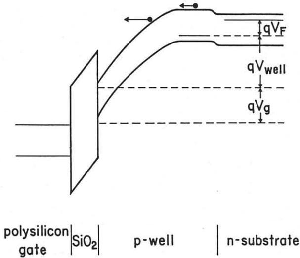
Fig. 2. Energy band diagram for injected electrons.
