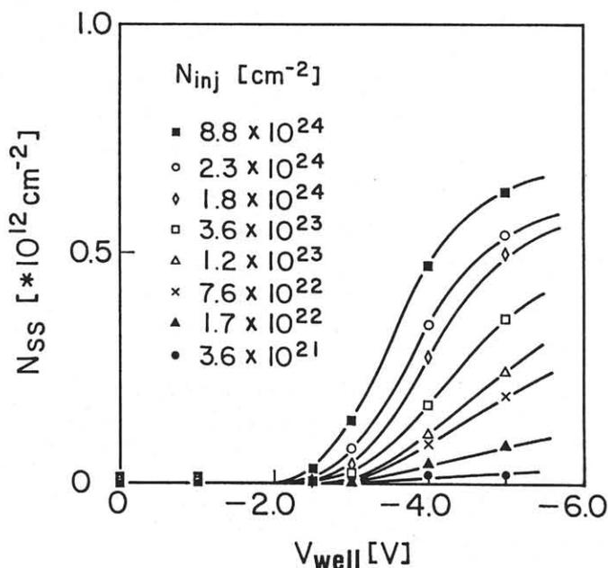
Fig. 5. Generated interface state density as a function of the p-well voltage. Stress gate voltage was 2.5 V.
