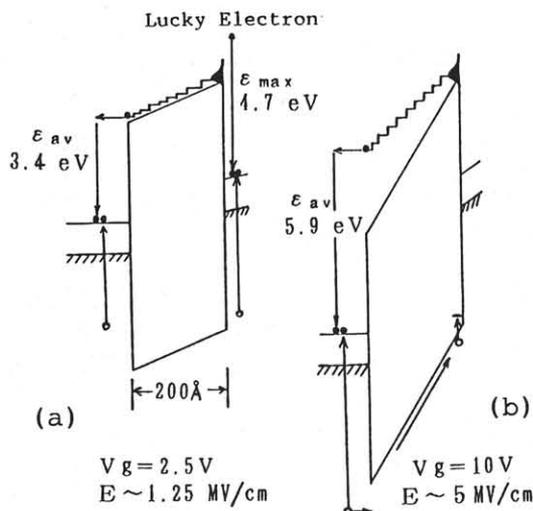
Fig. 4. Schematic illustration for two modes of interface state generation. The p-well voltage is  $-4.0$  V.
