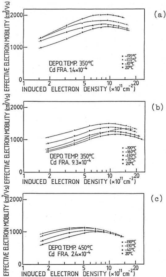
Fig.4 Effective mobility of electron as a function of  $N_s$  on the substrate with a parameter of the measuring temperature.
