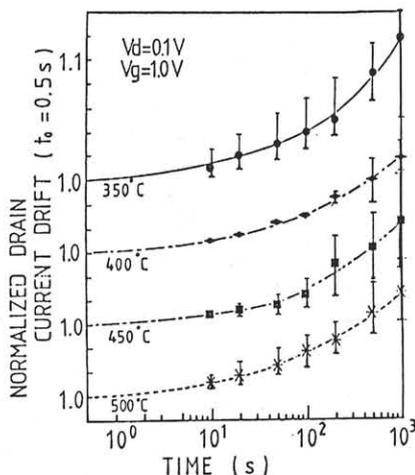
Fig.7 The drain current drift for the various vapor etching and PAsN deposition temperature.
