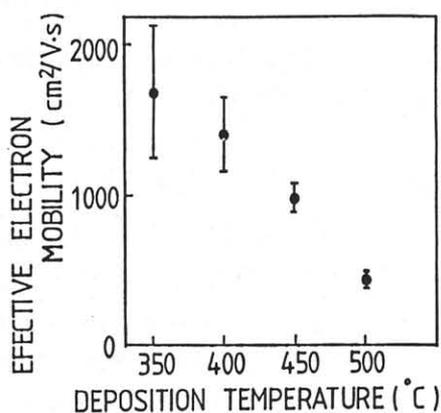
Fig.2 Effective mobility of electrons as a function of the vapor etching and PAsN deposition temperature.
