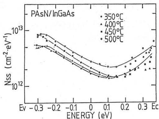
Fig.1 The density of interface trap states for various vapor etching and PAsN deposition temperature.
