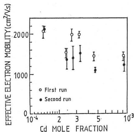
Fig.3 Effective mobility of electron as a function of Cd mole fraction in the melt from which the ingot for the substrate was grown.
