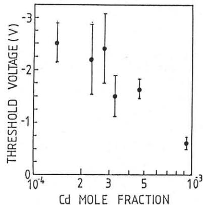
Fig.6 Threshold voltage as a function of Cd mole fraction in the melt.
