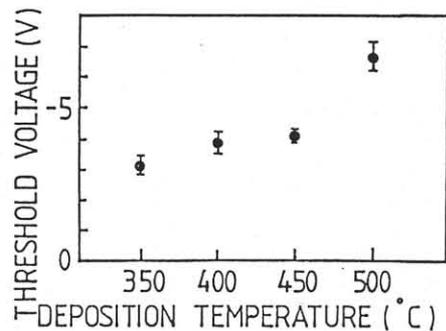
Fig.5 Threshold voltage as a function of vapor etching and PASN deposition temperature.
