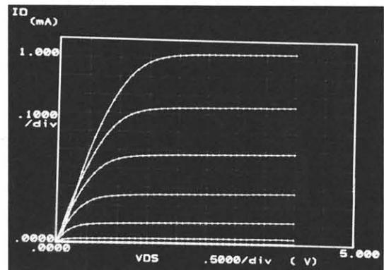
Fig.5  $I_d - V_d$  characteristics of a fabricated FET.  $V_g=+0.8\text{V} - 0.4\text{V}$  with 0.2V step.  $L_g/W_g=7\mu\text{m}/140\mu\text{m}$ .  $g_m=12\text{mS/mm}$  at  $V_g=+0.7\text{V}$  and  $K=0.80\text{mA/V}^2$ .
