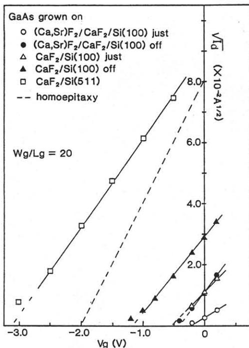
Fig.6  $\sqrt{I_d} - V_g$  characteristics of FET's fabricated on each structure and those on GaAs-homoepitaxial layer for comparison.
