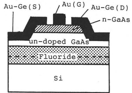
Fig.3 Schematic of a MESFET fabricated on a GaAs/fluoride/Si structure. The fluoride layer is  $(\text{Ca,Sr})\text{F}_2/\text{CaF}_2$  or  $\text{CaF}_2$ .
