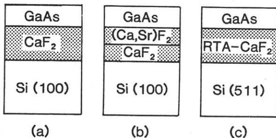
Fig.1 GaAs/fluoride/Si structures grown for FET fabrication in this work.
