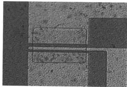
Fig.4 Optical micrograph of plan view of a fabricated MESFET of which cross-sectional structures is shown in Fig.3.  $L_g/W_g=3\mu\text{m}/60\mu\text{m}$ .
