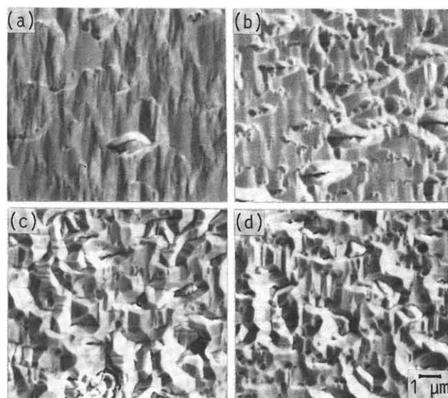
Fig.2 Surface morphologies of GaAs grown on fluoride/Si(100) structures. The fluoride layer and off-set angle of Si substrates are: (a) (Ca,Sr)F<sub>2</sub>/CaF<sub>2</sub>, 4°off (b) CaF<sub>2</sub>, 4°off (c) (Ca,Sr)F<sub>2</sub>/CaF<sub>2</sub>, just, (d) CaF<sub>2</sub>, just
