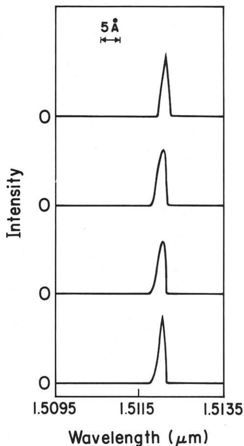
Fig. 6 Lasing spectra of SA-CM DFB laser array
