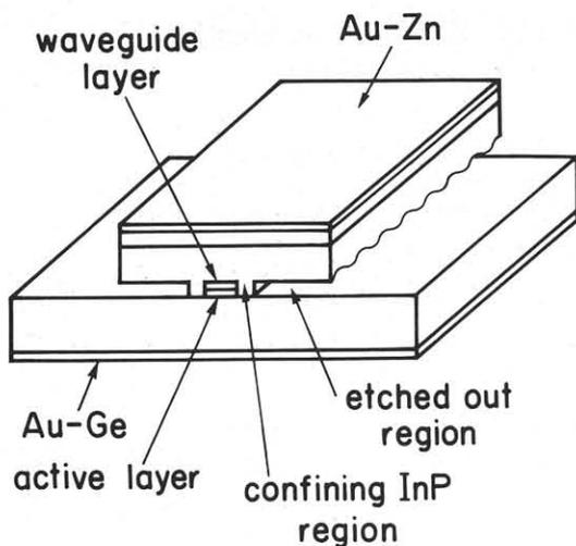
Fig. 1 Schematic structure of SA-CM DFB laser
