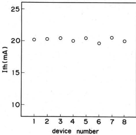
Fig. 4 Threshold currents of the lasers in the same bar
