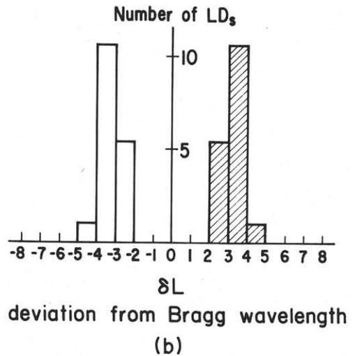
Fig. 5 Lasing wavelength distribution (a)experiment (b)theoretical calculation
