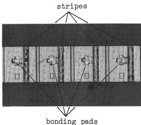
Fig. 2 Top view of SA-CM DFB laser array
