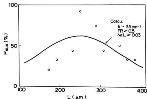
Fig. 3 Cavity length dependence of SLM probability
