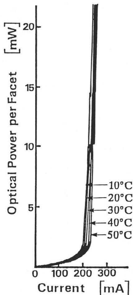
**Fig.2** Light output vs. injection current characteristics at different temperatures
