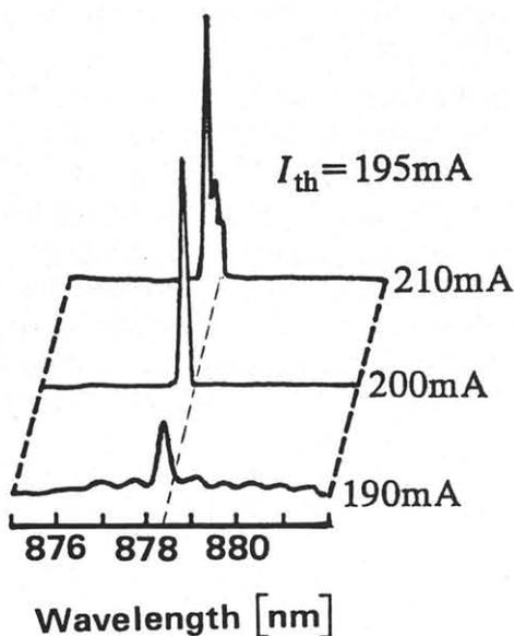
Fig.3 Injection current dependence of the lasing spectrum at 10°C
