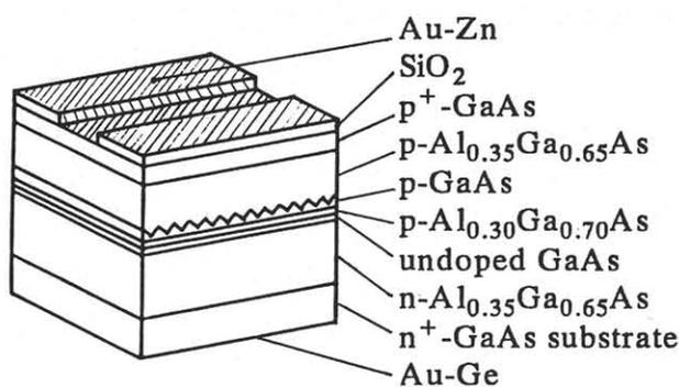
**Fig.1** Schematic drawing of the gain-coupled DFB laser diode with oxide stripe structure
