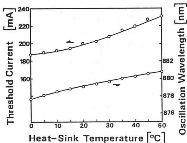
Fig.5 Dependence of the threshold current and the lasing wavelength on heat-sink temperature
