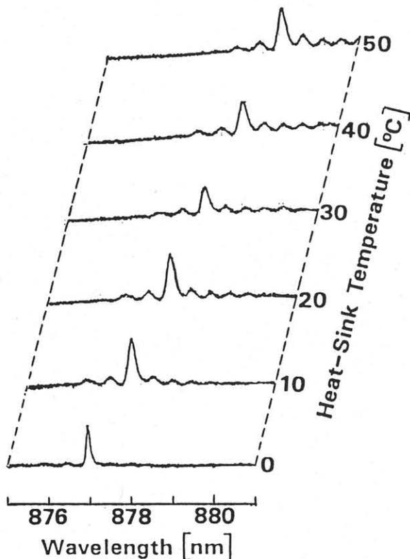
Fig.4 Near-threshold spectra at different temperatures
