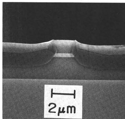
Fig.3 Cross sectional SEM photograph of end facet of TJ-BH MQW laser diode.
