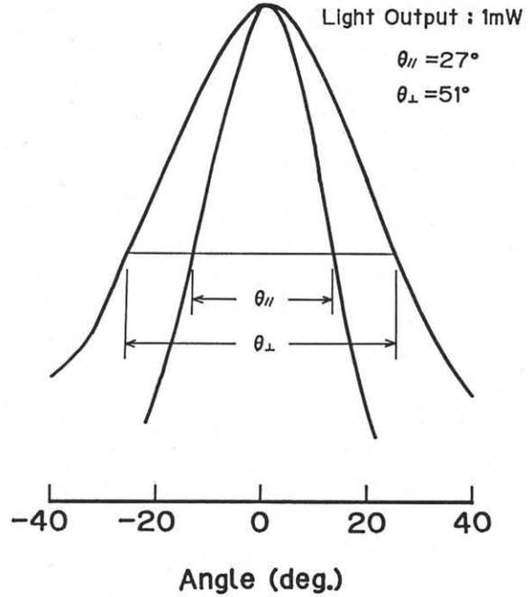
Fig.5 Far-field pattern of TJ-BH MQW laser diode at room temperature.
