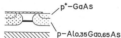
(5) Etching off  $\text{SiN}_x$  and Ohmic metalization
