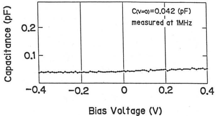
Fig.6 C-V characteristics of TJ-BH MQW laser diode at room temperature.
