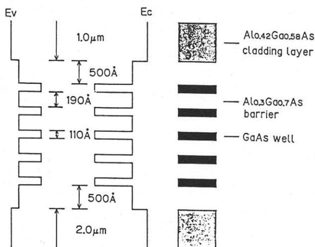
Fig.1 Schematic energy band diagram and structure of MQW.
