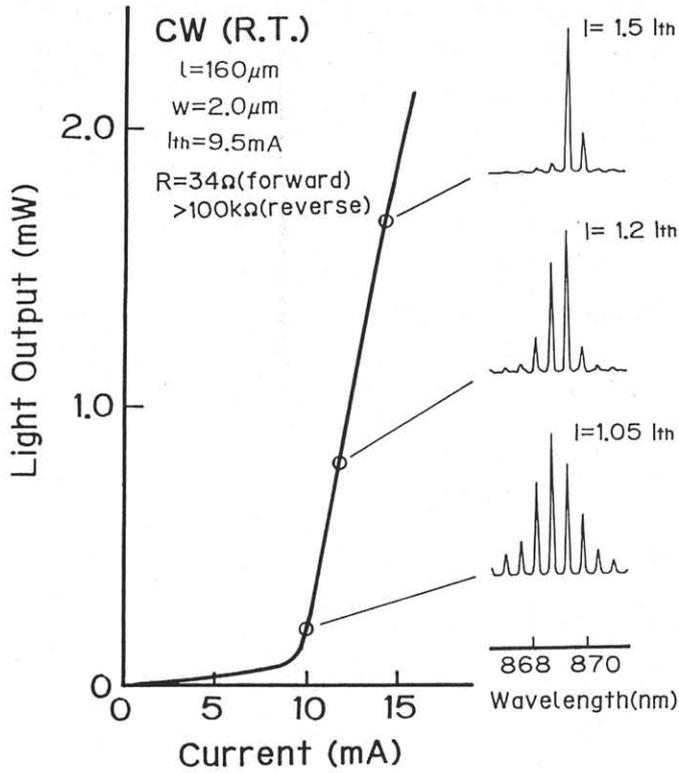
Fig.4 I-L characteristics of TJ-BH MQW laser diode under CW operation at room temperature; cavity length  $160\mu\text{m}$ .
