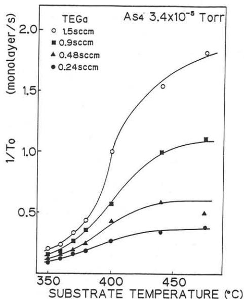
Fig.4. Dependence of  $1/T_0$  on the substrate temperature.
