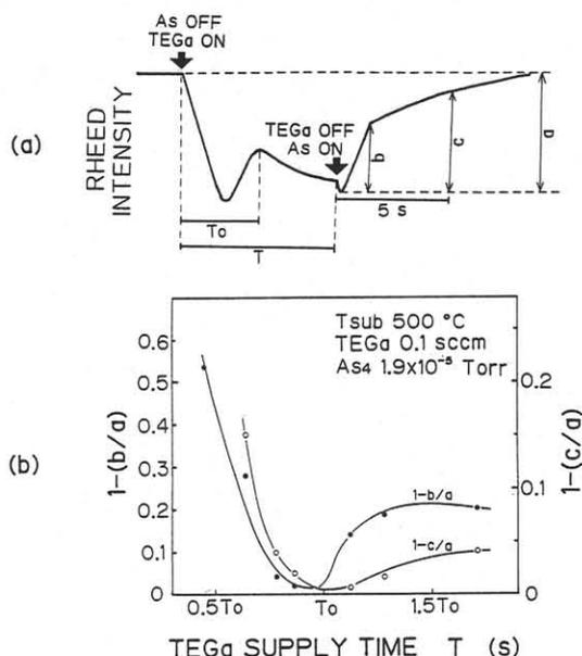
Fig.2. Recovery characteristic of RHEED intensity as a function of TEGa supply time. (a) RHEED intensity recovery after resupplying  $As_4$  molecules, and (b) recovery as a function of the TEGa supply time.
