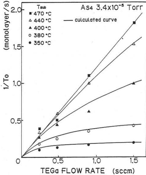
Fig.5. Dependence of  $1/T_0$  on the TEGa flow rate.
