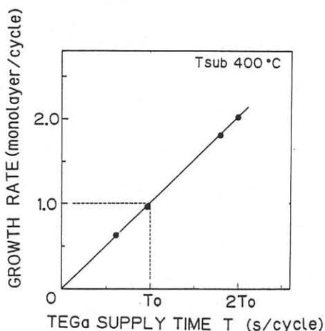
Fig.3. Growth rate per one cycle as a function of TEGa supply time.
