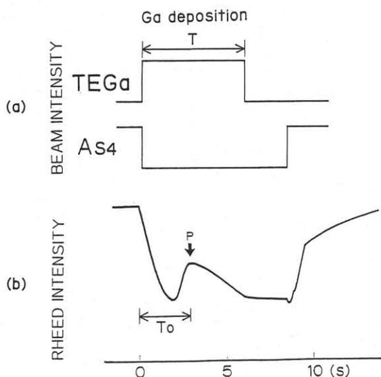
Fig.1. RHEED intensity variation during TEGa and  $As_4$  alternate supply. (a) shutter operation sequence, and (b) corresponding RHEED intensity variation.
