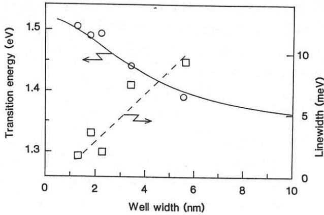
Fig.4 PL photon energies and full width at half maximum values of InGaAs/GaAs ( $x=0.25$ ) SQW samples. The solid line is the calculated curve based on the Kronig-Penny model. The dashed line is the visual guide for the FWHM values.
