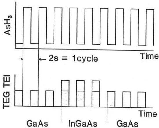
Fig.1 A gas flow sequence for fabricating SQW samples by flow-rate modulation epitaxy.
