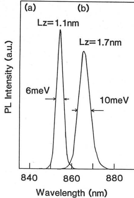
Fig.5 Low temperature (2 K) photoluminescence spectra of InGaAs/GaAs ( $x=0.45$ ) SQW samples. Well widths are (a) 1.1 nm and (b) 1.7 nm.
