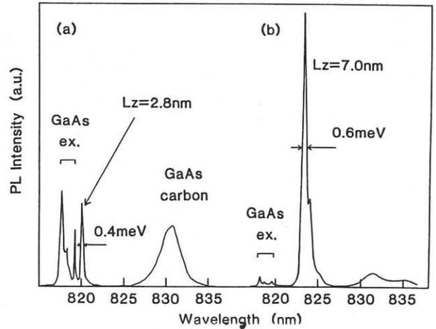
Fig.2 Low temperature (2 K) photoluminescence spectra of InGaAs/GaAs ( $x=0.063$ ) SQW samples. Well widths are (a) 2.8 nm and (b) 7.0 nm.
