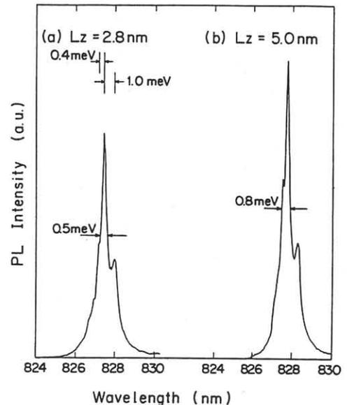
Fig.3 Low temperature (2 K) photoluminescence spectra of InGaAs/GaAs ( $x=0.063$ ) MQW samples. Well and barrier widths are (a) 2.8 nm and 2.5 nm, (b) 5.0 nm and 4.5 nm.
