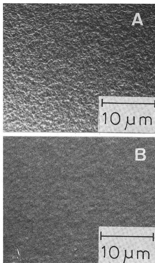
Fig. 1 Surface morphology: (A)  $T_s=250$  °C and (B)  $T_s=$ about 300 °C.
