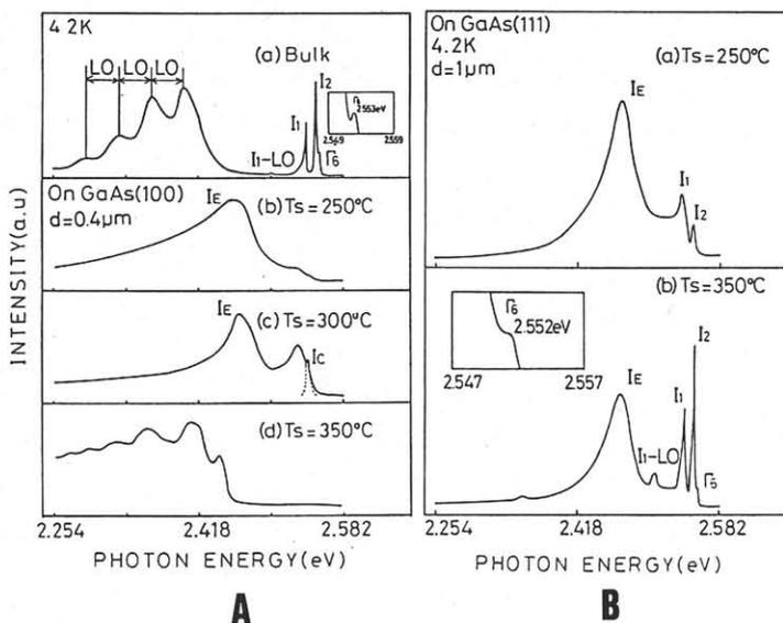
Fig. 3 PL spectra obtained at 4.2 K of CdS bulk and thin films: (A) (100) and (B) (111)A GaAs substrate.
