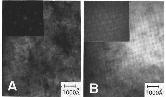
Fig. 5 TEM bright-field image and electron diffraction pattern of SLSs: (A) (100) and (B) (111)B GaAs substrate.
