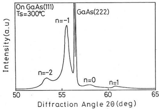
Fig. 4 X-ray diffraction spectrum of CdS (20 Å)-ZnS (42 Å) SLS grown on (111)A substrate.
