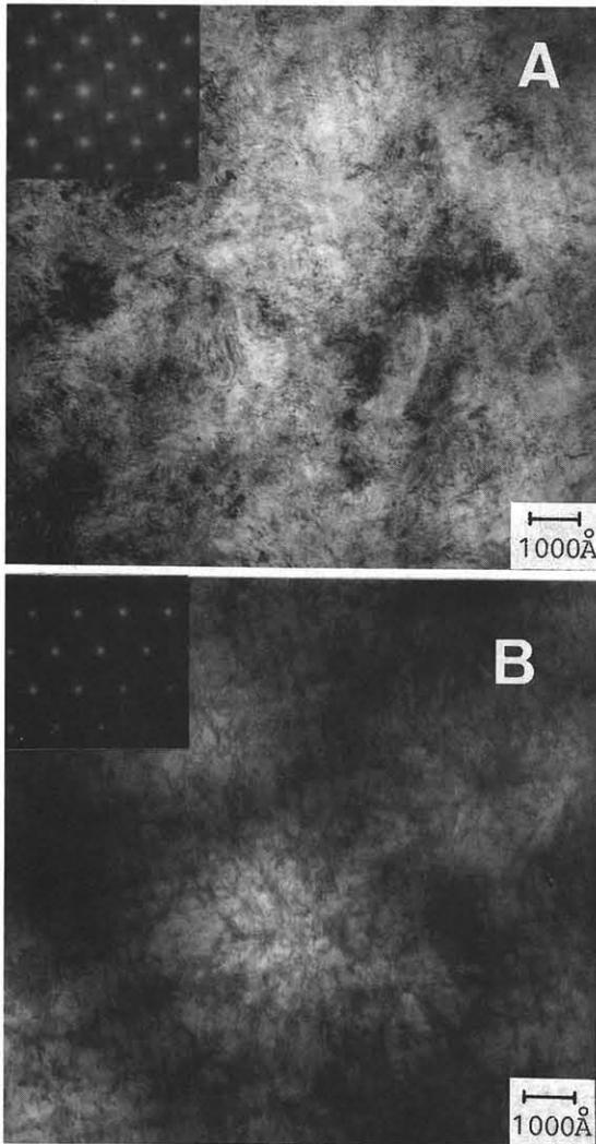
Fig. 2 Plan-view TEM bright-field image and electron diffraction pattern: (A) (100) and (B) (111)A substrate.
