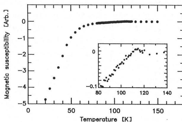
Fig.6 Temperature dependence of the magnetic susceptibility of Bi-Sr-Ca-Cu-O high- $T_c$  film. The detail around  $T_c$  is inserted.
