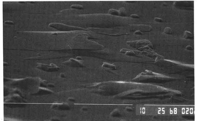
Fig.1 SEM of the Bi-Sr-Ca-Cu-O superconducting film after annealing. (Bar=10  $\mu m$ )
