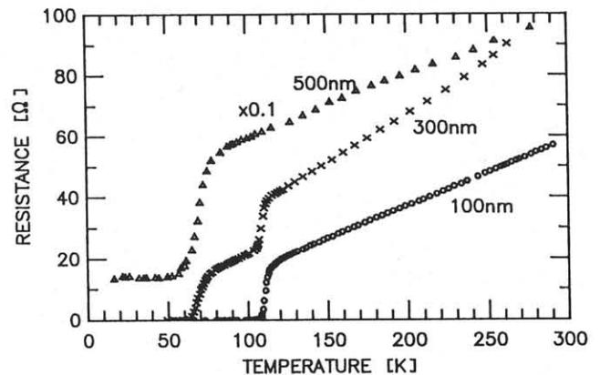
Fig.2 Temperature-resistance relation for various thickness samples of composition of 1212.
