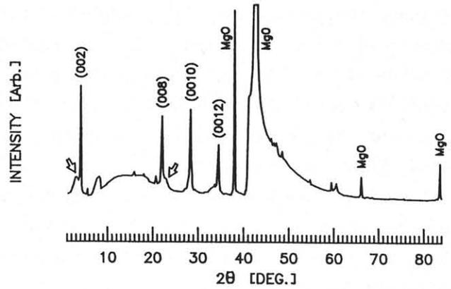
Fig.3 X-ray diffraction pattern of a typical high- $T_c$  film. The peaks indicated by arrows are unique to high- $T_c$  films.
