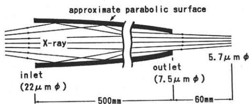
Fig. 2 Cross Section of X-ray Guide Tube made of Glass showing Principle of Focusing X-rays
