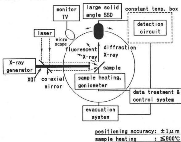
Fig. 1 Block Diagram of Focused X-ray Beam Spectrometer
