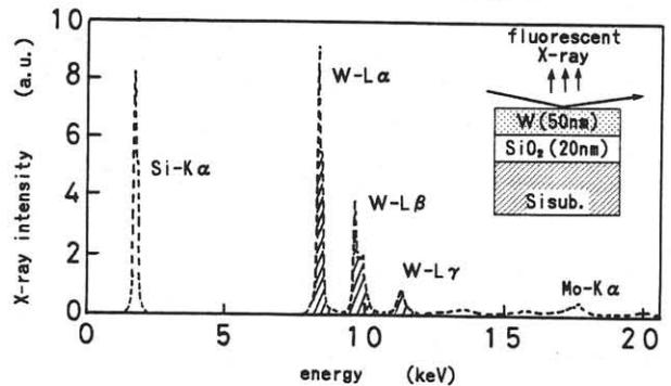
Fig. 4 Detection of W Fluorescent X-rays at Nearly Total Reflection Condition of Incident X-ray Beam
