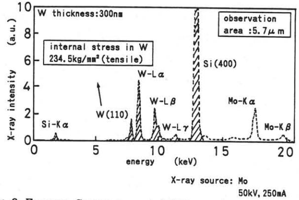
Fig. 3 Energy Spectrum of Diffraction X-rays and Fluorescent X-rays of W interconnect on Si-substrate
