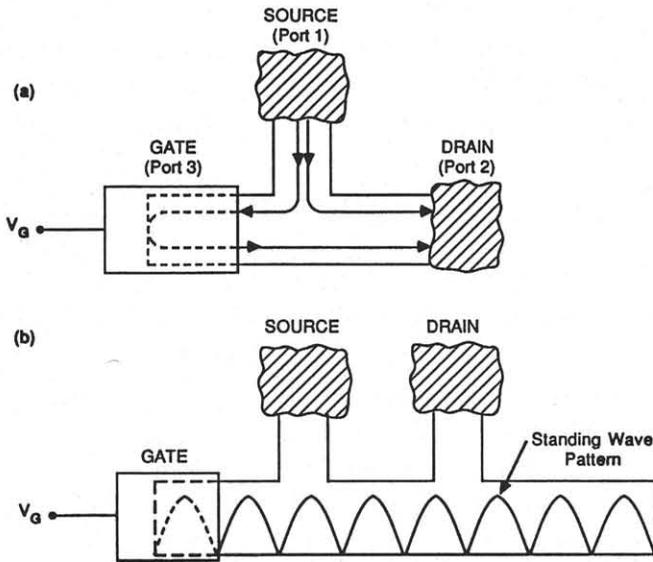
Fig. 2: Possible structures for quantum transistors with remote gates.
