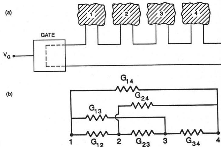
Fig. 3: A programmable multiterminal quantum network.
