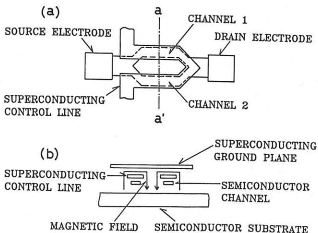
Fig.1. Proposed device structure. (a)Top view. (b)Cross sectional view along aa' line. The vertical structure is as follows: semiconductor channel/insulation layer/superconducting control line/insulation layer/ superconducting ground plane.
