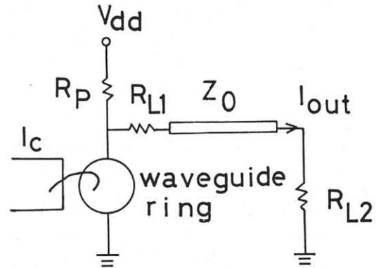
Fig.3. Proposed circuit configuration. The load resistance  $R_L$  is the sum of  $R_{L1}$  and  $R_{L2}$ . The strip line is terminated in the matching resistor  $R_{L2} = Z_0$ .  $V_{dd}$  is the source voltage, and  $R_p$  is the source resistor.
