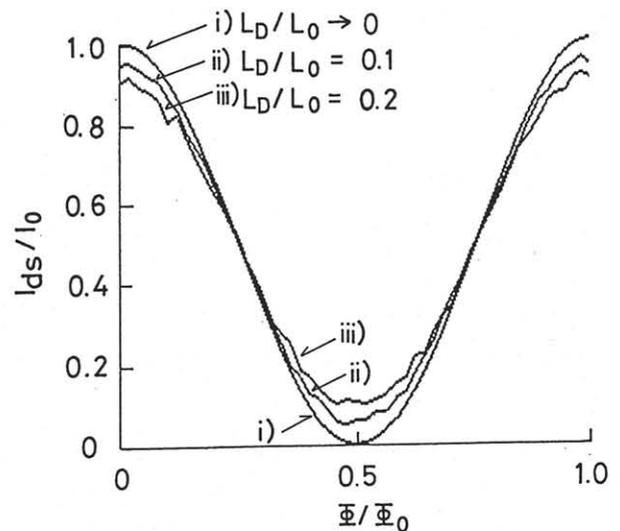
Fig.4. Calculated  $I_{ds}$  vs  $\Phi$  curves for different values of the ratio of  $L_D/L_0$ .
