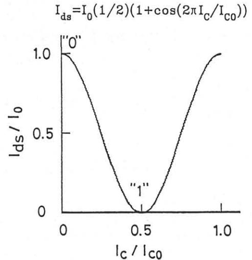
Fig.2.  $I_{ds}$  vs  $I_c$ . Here,  $I_{c0} = \Phi_0/M$ ,  $\Phi_0$  is a single flux quantum, and  $M$  is the mutual inductance.
