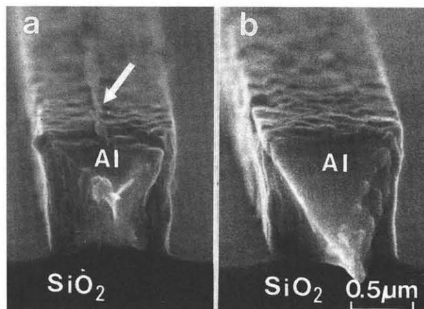
Fig. 4 Resist ashing after Al RIE. The ashing was implemented by the use of (a)  $\text{O}_2$  plasma and (b) reaction between fluorine atoms and water vapor, respectively.
