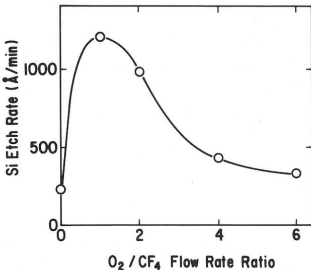
Fig. 5 Si etch rate vs.  $O_2$  to  $CF_4$  flow rate ratio.
