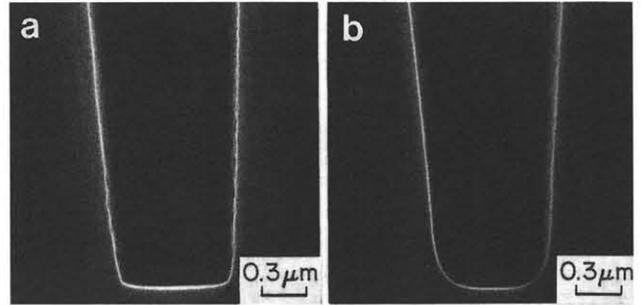
Fig. 6 Si trench features of (a) before and (b) after smoothing the roughened sidewall and rounding off the bottom corner with negative curvature, respectively.
