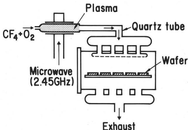
Fig. 1 Layout diagram of down-flow reactor.
