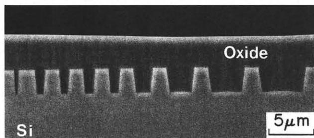
Fig. 8 Si trench feature after completely planarized with silicon oxide film at  $-40^\circ\text{C}$ .
