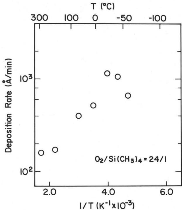
Fig. 7 Silicon oxide deposition rate vs. substrate temperature.
