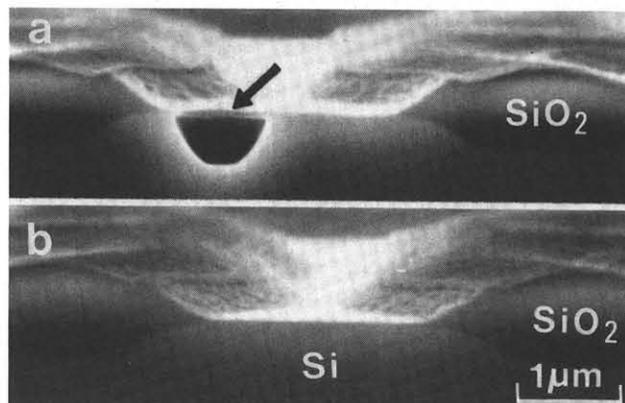
Fig. 3  $\text{Si}_3\text{N}_4$  removal in LOCOS.  $\text{Si}_3\text{N}_4/\text{SiO}_2$  selectivities are (a) 10 and (b) infinite, respectively.
