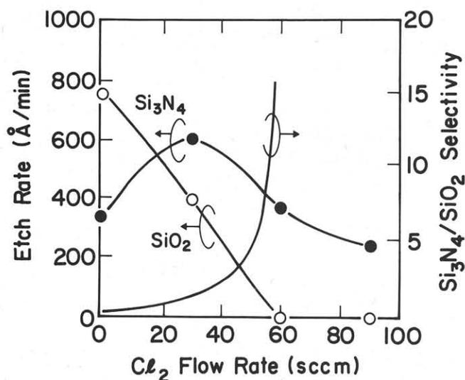
Fig. 2  $\text{Si}_3\text{N}_4$  and  $\text{SiO}_2$  etch rates vs.  $\text{Cl}_2$  flow rate at 30 sccm  $\text{NF}_3$ .
