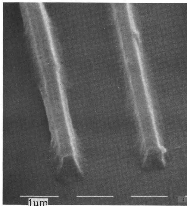
Fig.7 SEM photograph of 0.5 \mu\text{m} lines pattern of the new resist in 1.0 \mu\text{m} thickness.
