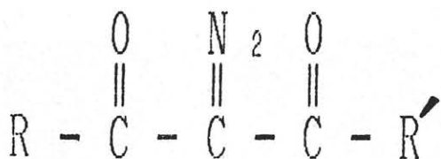
Fig.1 Chemical structure of the 2-diazo-1,3-dicarbonyl photoactive compound (R, R'; substituents).
