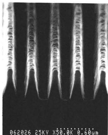
Fig.8 Undoped polysilicon patterns formed by  $\text{Cl}_2$  RIE.
