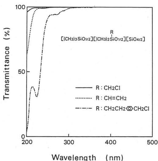
Fig.2 UV absorption spectra of the siloxane resists with different functional groups, R.
