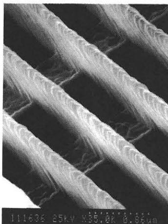
Fig.6 Bilayer resist patterns formed by O<sub>2</sub> RIE.
