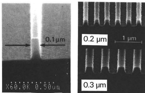
Fig.4 Siloxane resist patterns obtained by point-beam (left) and variable-shaped beam (right).
