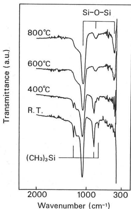
Fig.5 IR spectra of siloxane resist after annealing.
