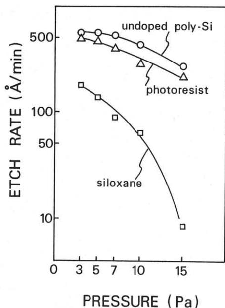
Fig.7  $\text{Cl}_2$  gas pressure dependence of etching rates for various materials.
