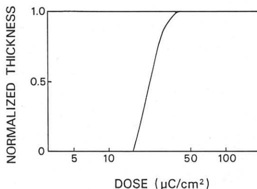
Fig.3 Sensitivity curve of the siloxane resist.
