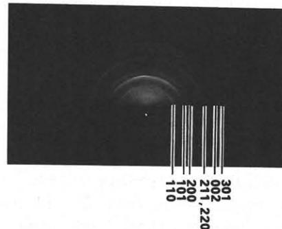
Fig. 9 RHEED pattern from Si surface after removals of W and TiN.
