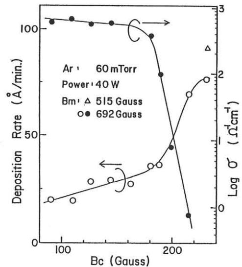
Fig.4 Bc dependences of deposition rate and logarithmic conductivity.
