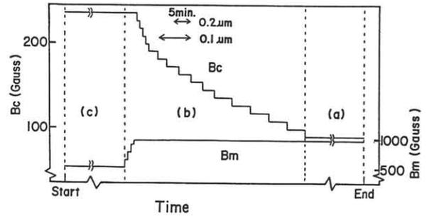
Fig.5 Time variation of  $B_c$  and  $B_m$  to deposit compositional gradient film by controlling plasma area on the target.
