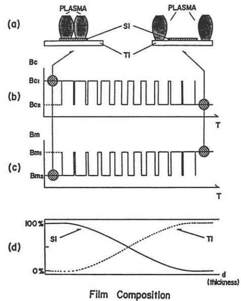
Fig.6 Duty ratio variation of  $B_c$  and  $B_m$  to deposit compositional gradient film.
