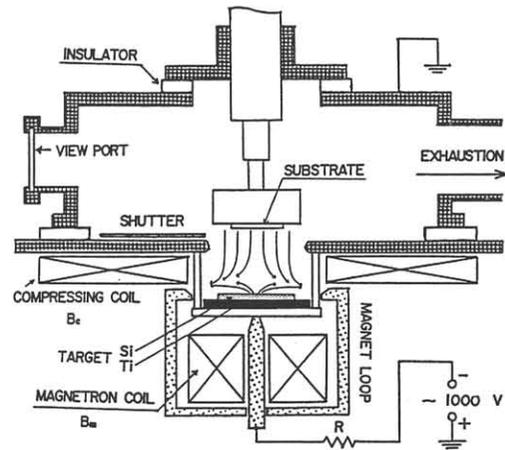
Fig.1 Chamber of plasma controlled sputtering.
