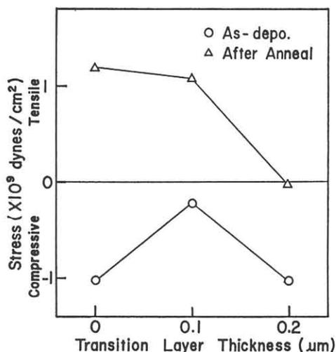
Fig.8 Stresses before and after annealing for various thickness of transition layers.
