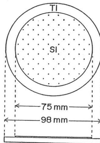
Fig.2 Target configuration of composition control.
