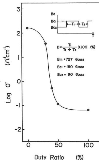
Fig.7 Relation between  $\text{Log } \sigma$  of  $TaSi_x$  and duty ratio.
