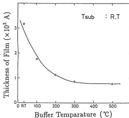
Fig.3 SiO<sub>2</sub> film thickness as a function of the buffer temperature at wafer temperature  $T_{\text{sub}}=R.T.$
