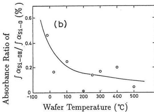
Fig.4 (a)  $\text{SiO}_2$  film thickness and (b) ratio of integral absorption coefficient for Si-OH to Si-O bonds as a function of wafer temperature at buffer temperature  $T_{\text{buf}}=400^\circ\text{C}$ .
