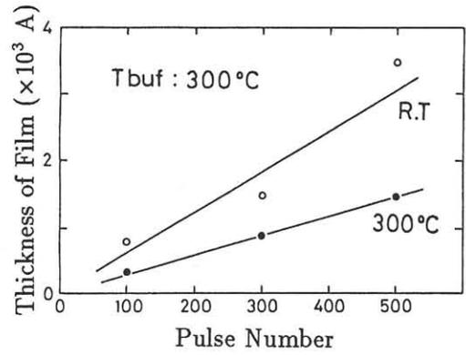
Fig.6  $\text{SiO}_2$  film thickness as a function of number of pulse at buffer temperature  $T_{\text{res}}=300^\circ\text{C}$ .
