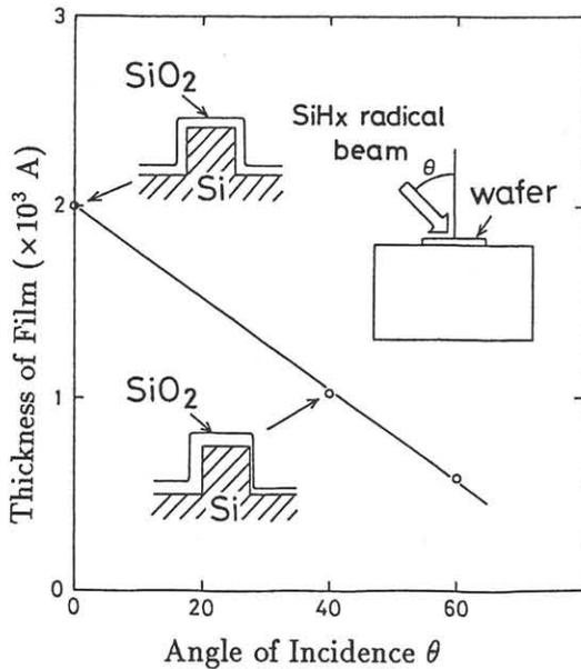
Fig.7 Film thickness and cross-sectional illustration of  $\text{SiO}_2$  as a function of an incidence angle of  $\text{SiH}_x$  radicals.
