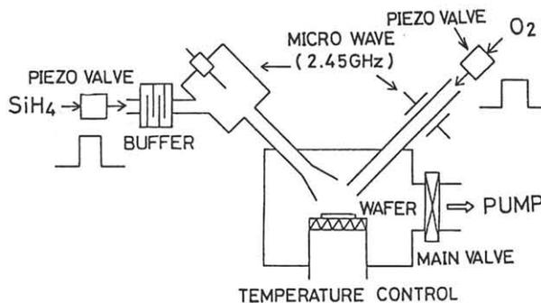
Fig.1 A schematic illustration of the digital CVD apparatus.
