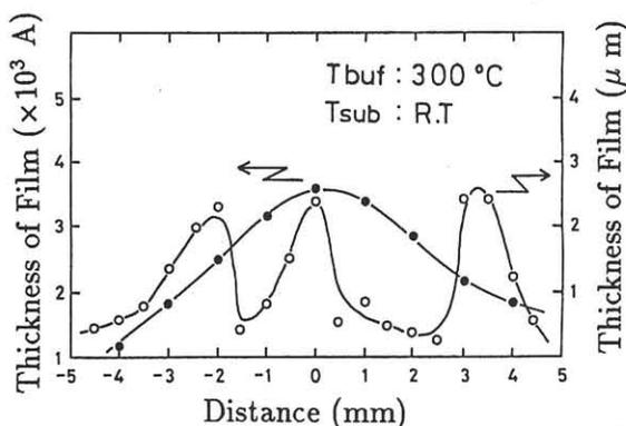
Fig.2 Deposition profiles in the cases with and without the buffer at buffer temperature  $T_{\text{buf}}=300^\circ\text{C}$  and wafer temperature  $T_{\text{sub}}=300^\circ\text{C}$ .
