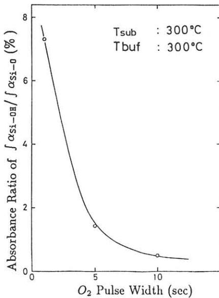
Fig.5 Ratio of integral absorption coefficient for Si-OH to Si-O bonds as a function of pulse width of  $\text{O}_2$  gas at buffer temperature  $T_{\text{buf}}=300^\circ\text{C}$  and wafer temperature  $T_{\text{sub}}=300^\circ\text{C}$ .
