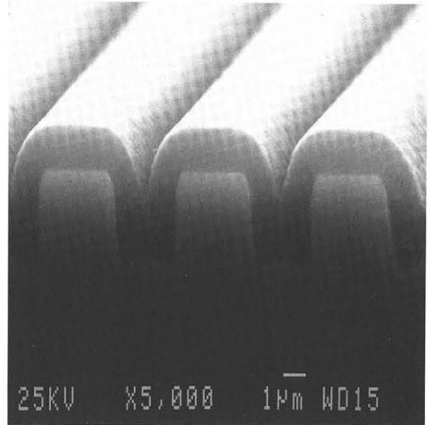
Fig.8 Cross-sectional SEM photograph of  $\text{SiO}_2$  film filled in the trench with aspect ratio of 2.
