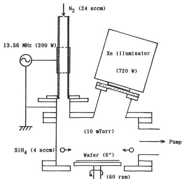
Fig.1. Schematic of PAP-CVD apparatus.
