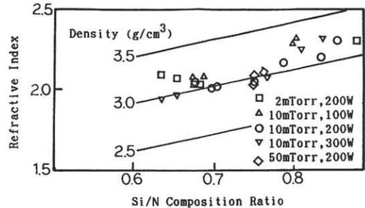
Fig.6. Refractive index vs. Si/N composition ratio.
