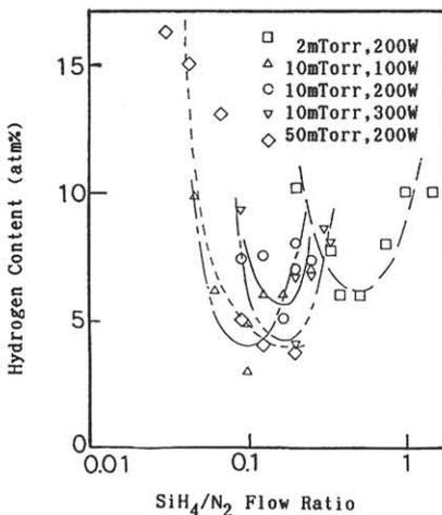
Fig.4. Hydrogen content vs.  $\text{SiH}_4/\text{N}_2$  flow ratio.
