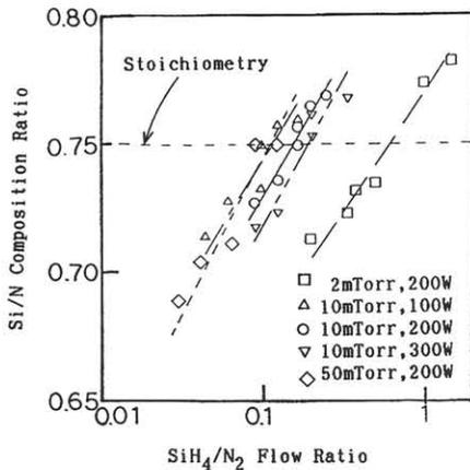
Fig.3. Si/N composition ratio vs.  $\text{SiH}_4/\text{N}_2$  flow ratio.
