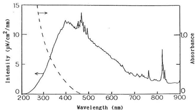
Fig.2. Emission spectrum of Xe illuminator (—) and absorption spectrum of reactive intermediates(---).
