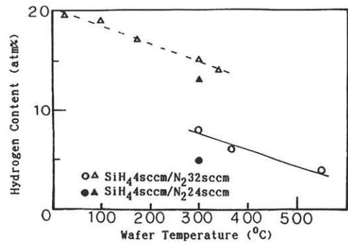
Fig.5. Hydrogen content vs. wafer temperature with Xe irradiation(—) or resistive heating(---).
