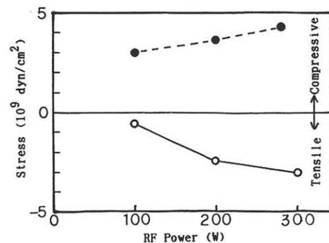
Fig.7. Stress vs. RF power with(—) or without(---) irradiation.
