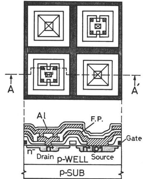
Fig. 3 The proposed cell structure for a high-voltage MOSFET.
