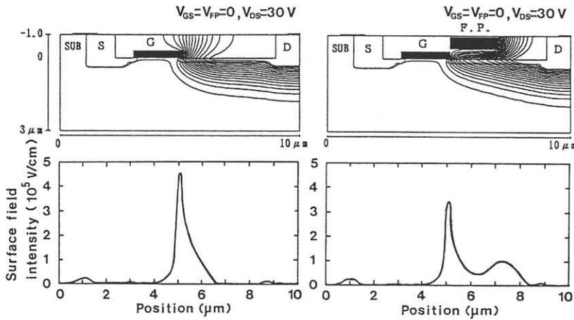
(a) without a field plate. (b) with a field plate.
