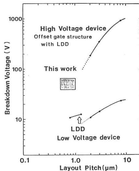
Fig. 1 The relationship between breakdown voltages and design rules for high and low-voltage MOSFETs.
