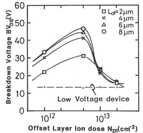
Fig. 5 Experimental results for breakdown voltages of the fabricated devices.
