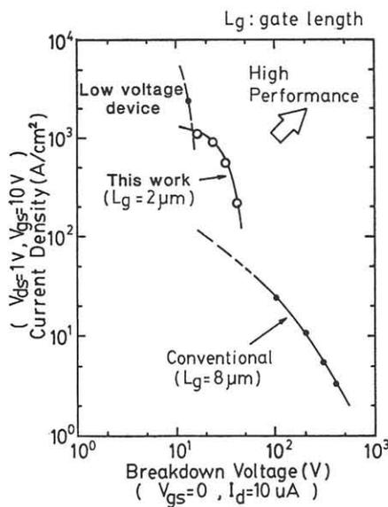
Fig. 6 Relationship between normalized current density and breakdown voltage.
