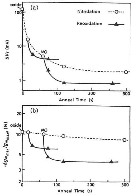
Fig. 9. (a)  $V_T$  shift and (b)  $g_{mmax}$  degradation after fixed products (substrate current  $\times$  stress time) of 1 and 0.1 C, respectively, as a function of anneal time for nitridations at 950  $^{\circ}C$  and subsequent reoxidations at 1150  $^{\circ}C$ .
