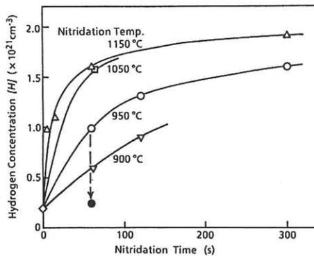
Fig. 2. Hydrogen concentration  $[H]$  measured by SIMS versus nitridation time. A dashed arrow and ● indicate the effect of reoxidation of  $NO$  at 1150 °C for 60 s.
