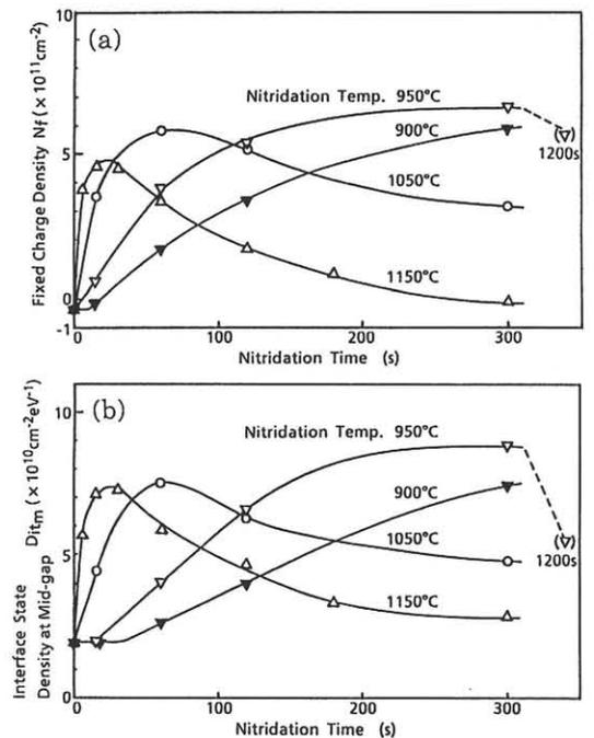
Fig. 3. (a) Fixed charge density  $N_f$  and (b) midgap interface state density  $D_{itm}$  versus nitridation time.
