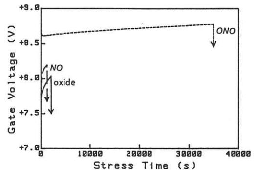
Fig. 4. Gate voltage to maintain a constant-current stress at 10 mA/cm<sup>2</sup> versus stress time. Arrows indicate breakdown times.
