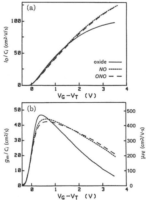
Fig. 7. (a) Drain current  $I_D$  and (b) transconductance  $g_m$  normalized by insulator capacitance  $C_i$  versus gate drive  $V_G - V_T$  for large-geometry MOSFET's with SiO<sub>2</sub>, NO, and ONO. Field-effect mobility  $\mu_{FE}$  is also shown in Fig. (b). The measured  $V_D$  was 0.1 V.
