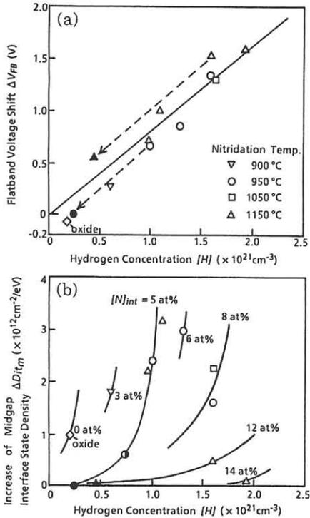
Fig. 6. (a)  $\Delta V_{FB}$  and (b)  $\Delta D_{itm}$  induced by  $0.1\text{-C}/\text{cm}^2$  electron injection versus hydrogen concentration  $[H]$ .  $\odot$  and  $\bullet$  ( $\triangle$  and  $\blacktriangle$ ) in these figures are the data for NO (NO<sub>HT</sub>) reoxidized for 60 s at 1050 and 1150 °C, respectively.
