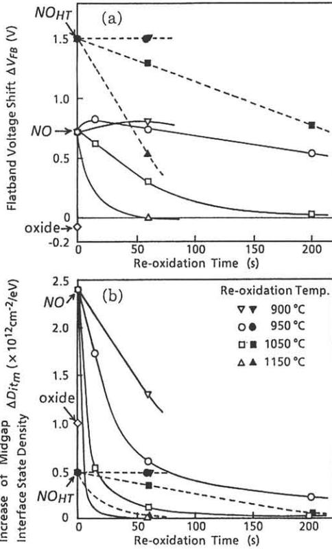
Fig. 5. (a) Flatband voltage shift  $\Delta V_{FB}$  and (b) increase of midgap interface state density  $\Delta D_{itm}$  induced by  $0.1\text{-C}/\text{cm}^2$  electron injection versus reoxidation time. The starting nitrated oxides are NO (lightly nitrated at 950 °C for 60 s) and NO<sub>HT</sub> (heavily nitrated at 1150 °C for 60 s).
