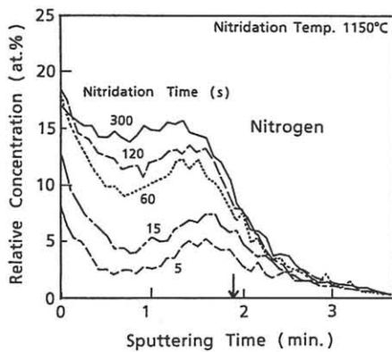
Fig. 1. Nitrogen AES depth profiles of oxides nitrided for various nitridation times at 1150 °C. An arrow indicates the position of the Si-SiO<sub>2</sub> interface.
