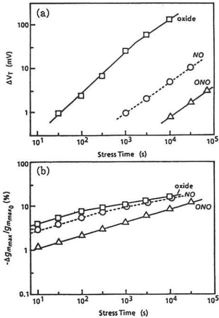
Fig. 8. (a) Threshold voltage shift  $\Delta V_T$  and (b) degradation of maximum transconductance  $-\Delta g_{mmax}/g_{mmax0}$  as a function of stress time for 0.8- $\mu$ m MOSFET's with  $SiO_2$ , NO, and ONO. The stress condition was  $V_D/V_G = 6 V/2 V$ .
