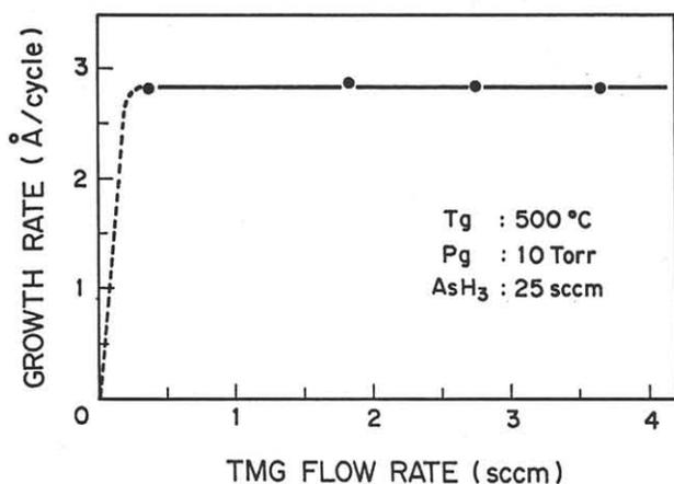
Fig.4 Growth rate as a function of TMG flow rate for nonirradiated growth
