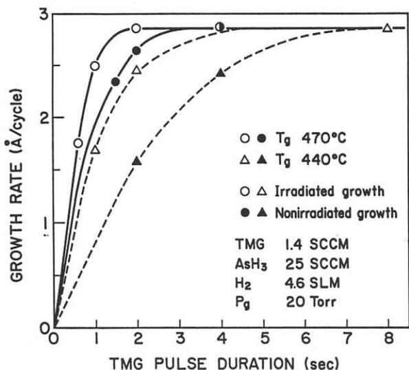
Fig.3 Growth rate as a function of TMG pulse duration for laser irradiated growth and nonirradiated growth
