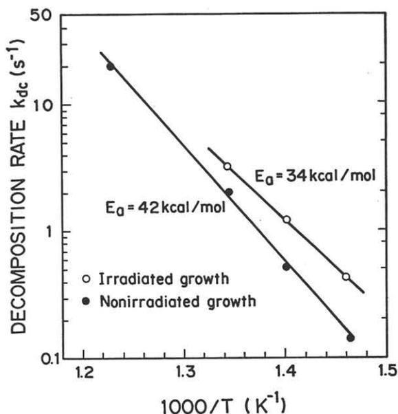
Fig.5 Decomposition rate  $k_{dc}$  for TMG on the surface, as a function of growth temperature
