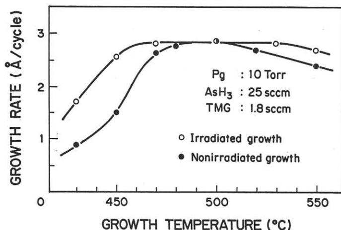
Fig.2 Growth rate as a function of growth temperature for laser irradiated growth
