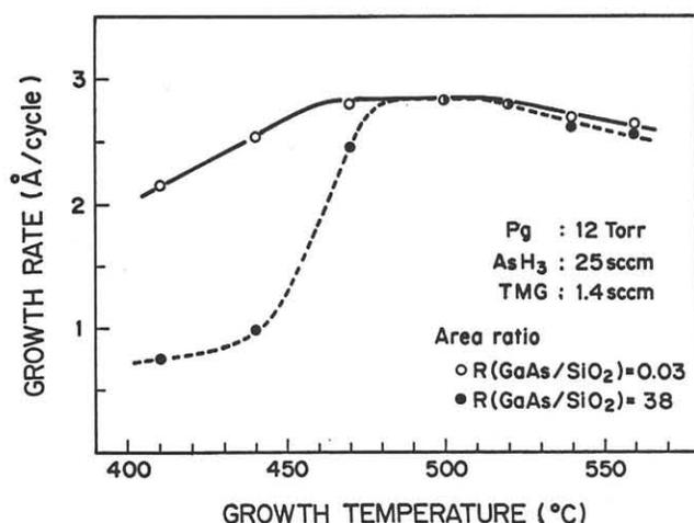
Fig.6 Growth rate temperature dependence for two substrate with different pattern configurations
