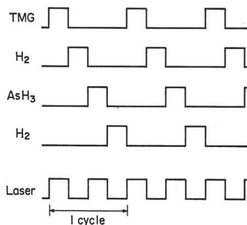
Fig.1 Time sequences for gases and laser irradiation
