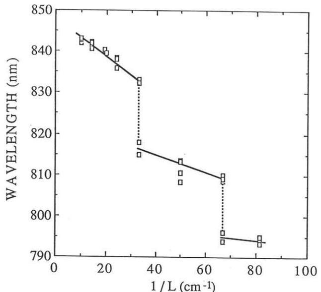
**FIG.2.** Lasing wavelength at the lasing threshold as a function of the reciprocal of the cavity length.
