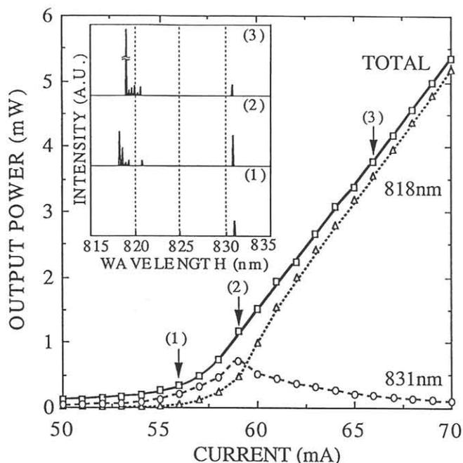
**FIG.3.** Output power vs. injection current characteristics of the ADQW LD with 301 $\mu m$  cavity length under CW operation at 5°C. The output power of 831nm light (circles) and 818nm light (triangles) are shown as well as the total power (squares). The emission spectra at three different injection levels are also shown in the inset.
