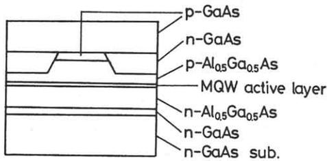
Fig.1 Schematic cross section of planar-buried ridge stripe structure
