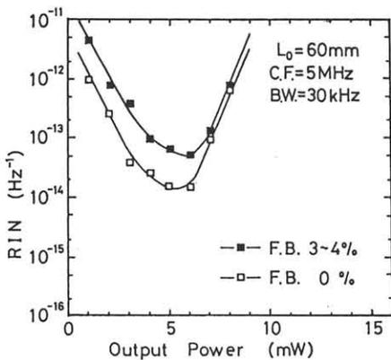
Fig.5 Relative intensity noise vs. light output power
