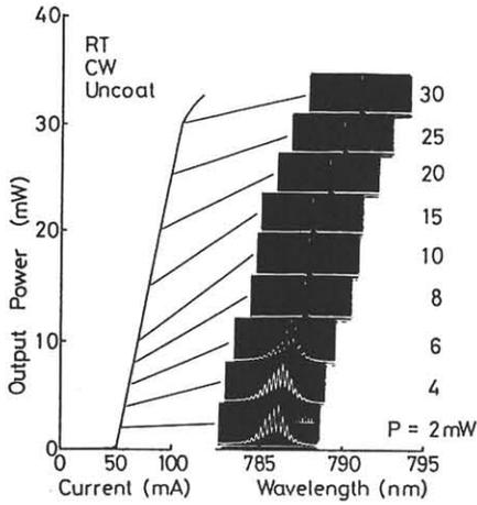
Fig.4 Light output power vs injected current characteristics and the longitudinal-mode spectra of the MQW laser
