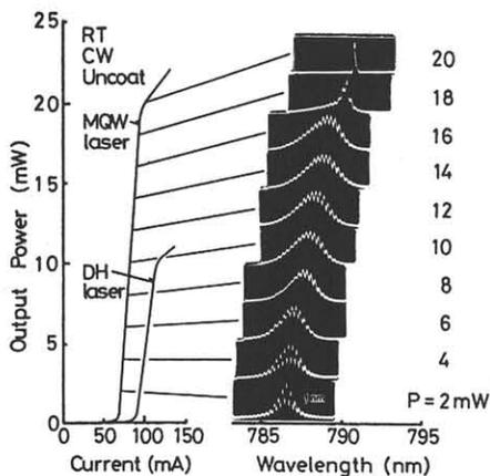
Fig.2 Light output power vs injected current characteristics of the MQW and DH lasers and the longitudinal-mode spectra of the MQW laser
