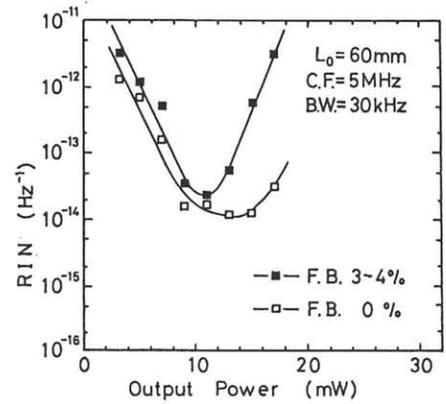
Fig.3 Relative intensity noise vs. light output power
