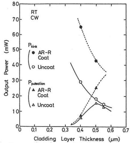
Fig.6 Dependence of kink levels and the maximum powers where self-sustained pulsation are observed on the cladding layer thickness
