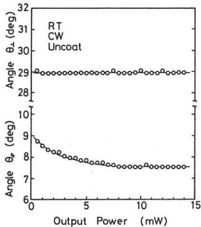
Fig.7 Dependence of FWHM perpendicular and parallel to the junction on the output power
