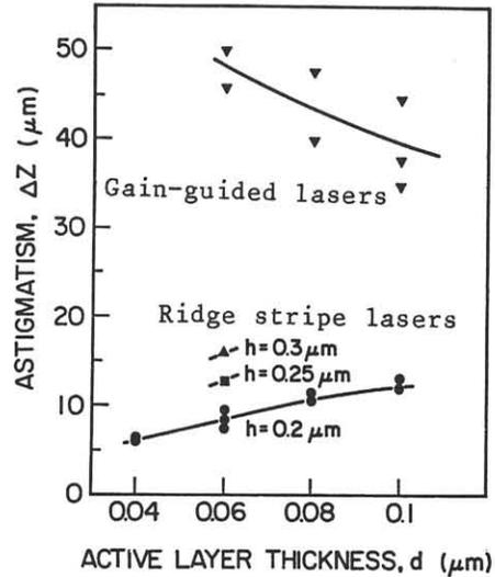
Fig. 3 Measured astigmatism dependence on the active layer thickness
