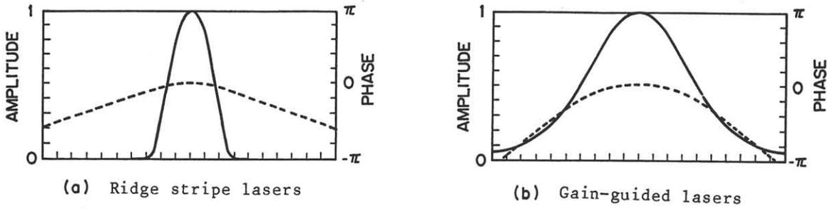
Fig. 2 Waveguide mode profiles for InGaAlP laser diodes
