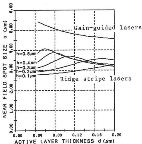
Fig. 5 Calculated spot size dependence on active layer thickness
