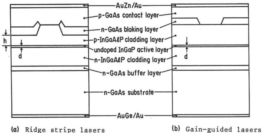
Fig. 1 Cross-sectional view of InGaAlP laser diodes
