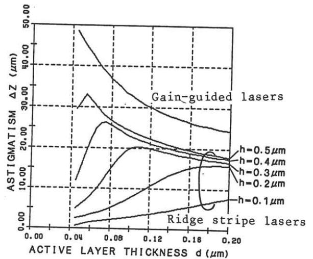
Fig. 4 Calculated astigmatism dependence on active layer thickness
