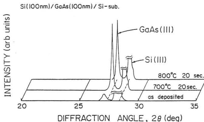
Fig.2 The X-ray diffraction patterns for poly-Si/GaAs/Si layered films annealed at different temperatures.
