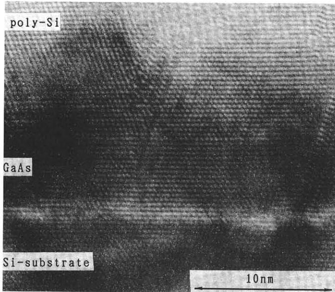
Fig.3 The TEM cross-section of the layered structure.
