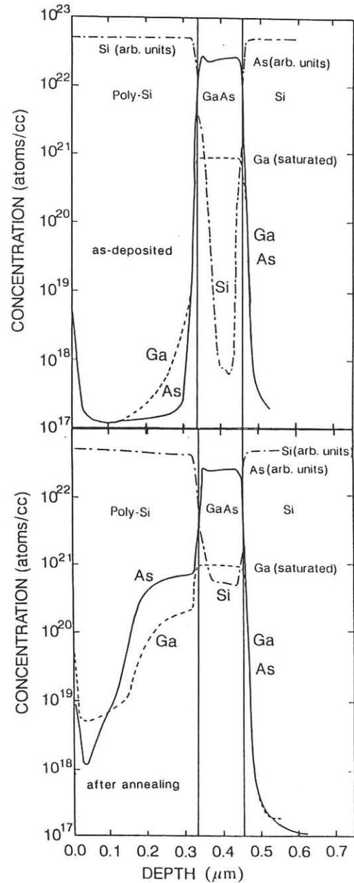
Fig.4 The impurity profiles in the layered structure.
