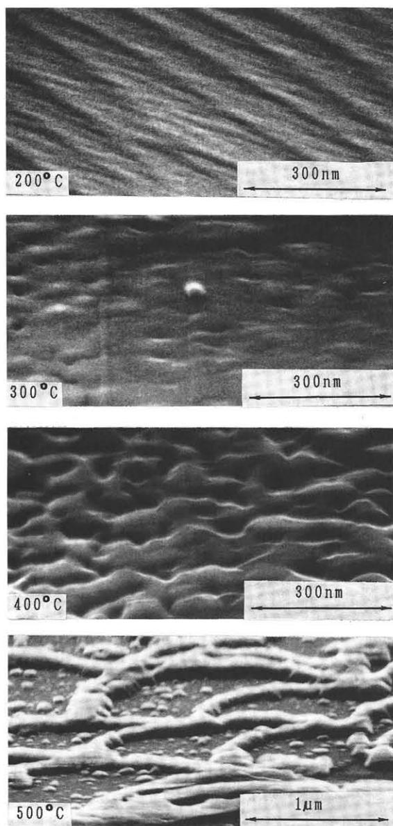
Fig.1 The surface morphology of GaAs films on Si deposited at different growth temperatures.
