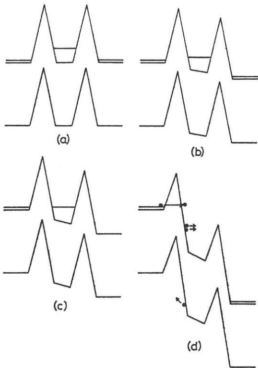
Fig.3 The band diagram (a) at thermal equilibrium, (b) at very low bias, (c) under resonant tunneling condition, (d) under impact avalanche breakdown.
