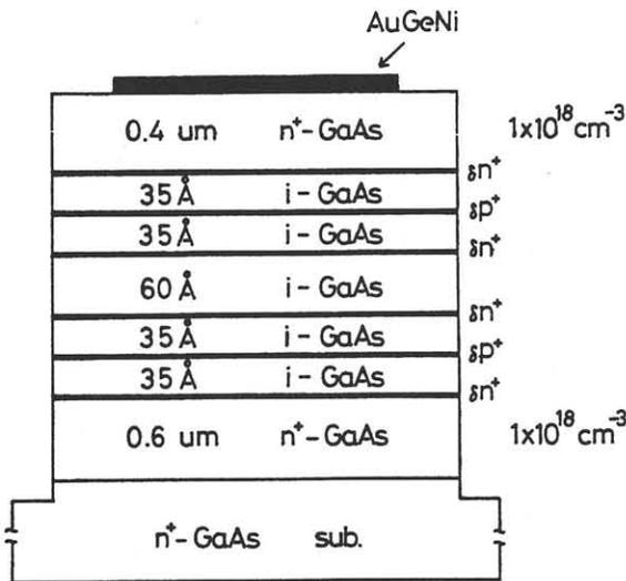
Fig.1 The schematic cross-section of the device structure with  $\delta n^+$  and  $\delta p^+$  concentrations  $2.5 \times 10^{13} \text{ cm}^{-3}$  and  $5 \times 10^{12} \text{ cm}^{-3}$ , respectively.
