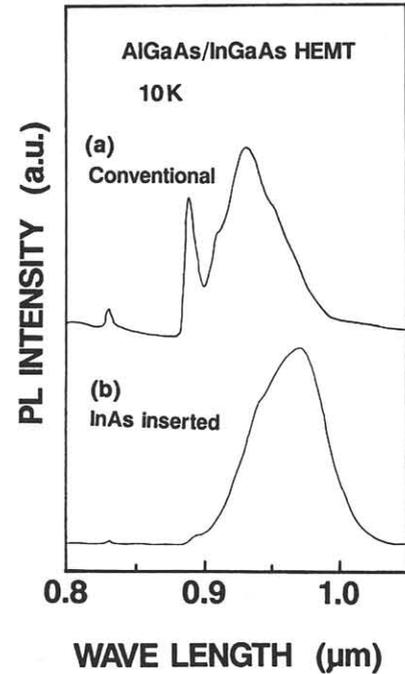
Fig. 6 Photoluminescence spectra from AlGaAs/InGaAs pseudomorphic HEMT at 10K. (a) and (b) indicate a conventional and a newly designed wafer, respectively.
