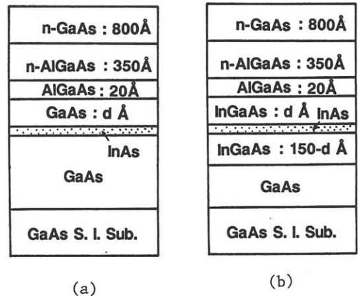
Fig. 3 Wafer structures of a newly developed HEMT. (a)  $\text{AlGaAs}/\text{GaAs}$  system, (b)  $\text{AlGaAs}/\text{InGaAs}$  system.
