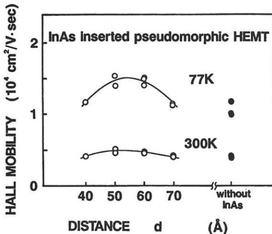
Fig. 5 The correlation between an InAs monolayer position and maximum Hall mobility for an AlGaAs/InGaAs HEMT structure.
