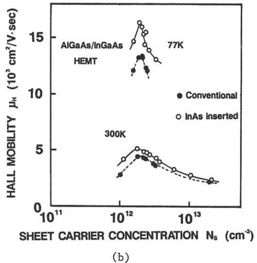
Fig. 4 The correlation between Hall mobility  $\mu_H$  and sheet density  $N_s$ . (a) AlGaAs/GaAs system, (b) AlGaAs/InGaAs system. The open circle indicates a new HEMT wafer with an InAs layer ( $d=50\text{A}$ ), and the closed circle indicates a conventional HEMT wafer.
