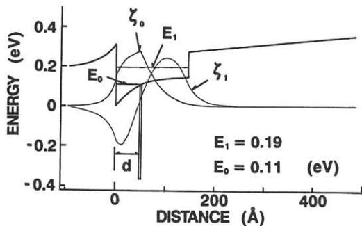
Fig. 2 The wave function, the self-consistent potential and the subband energy of a new pseudomorphic HEMT wafer with an  $\text{InAs}$  monolayer ( $d=50\text{\AA}$ ). "d" is the distance between the  $\text{AlGaAs}/\text{InGaAs}$  interface and the  $\text{InAs}$  monolayer.
