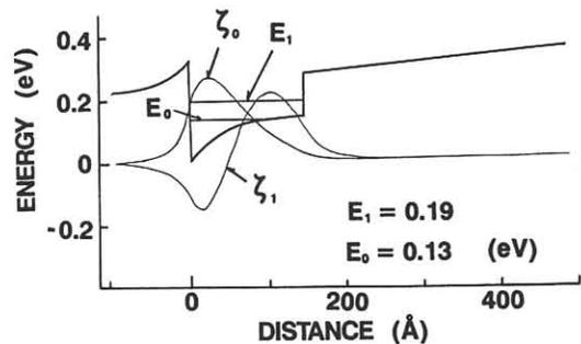
Fig. 1 The wave function, the self-consistent potential and the subband energy of a conventional pseudomorphic HEMT wafer.  $\zeta_0$  and  $\zeta_1$  represent the envelope wave functions of electrons in the two lowest subbands.  $E_0$  and  $E_1$  indicate the two lowest subband energies from the bottom of the InGaAs conduction band at the AlGaAs/InGaAs interface.
