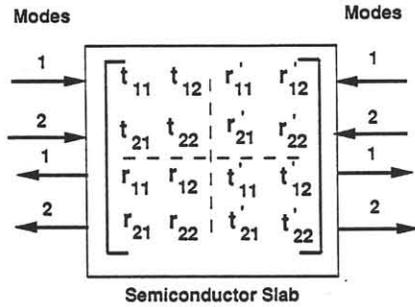
Fig. 2 The figure shows scattering matrix across a slab of semiconductors with 2 incoming and 2 outgoing modes.
