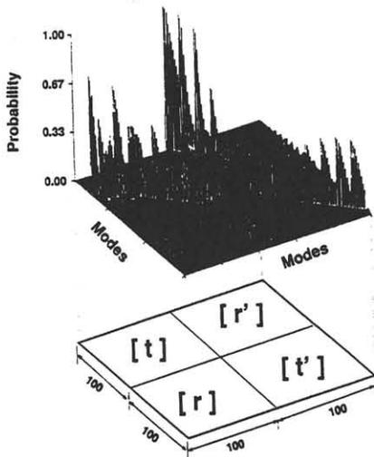
Fig. 3 A sample scattering matrix with 100 modes computed using a Monte Carlo simulator [2].
