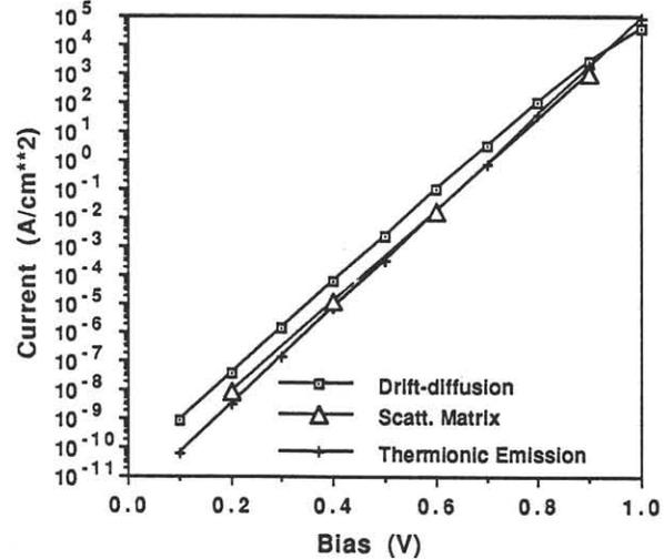
Fig. 5 Current-voltage characteristics of an M-S diode.
