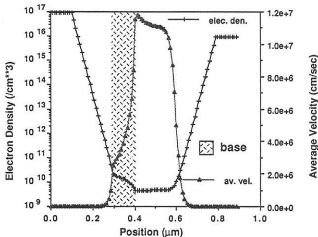
Fig. 6 The figure shows the average velocity and electron density versus position across a model transistor structure.
