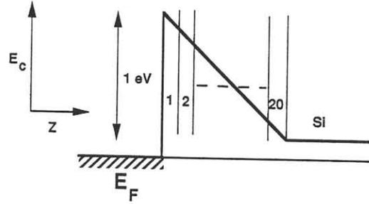
Fig. 4 Band diagram of an M-S diode. 20 scattering matrices are used.
