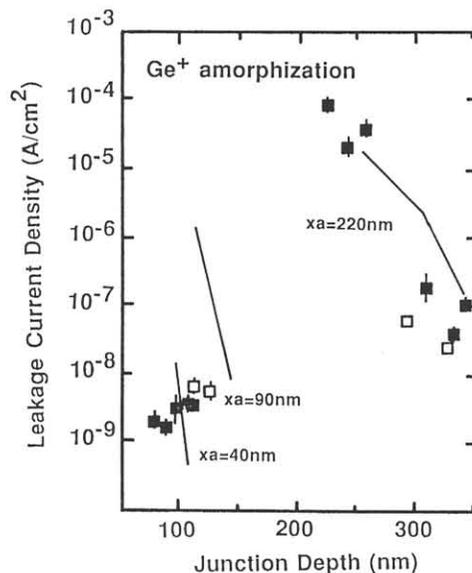
Fig.2 Variation of leakage current density for  $\text{Ge}^+$  pre-amorphized samples. Closed squares and open squares indicate the present and previous data, respectively. Solid lines indicate  $J_l^{\text{model}}=C/m \int N_{\text{int}}(x) dx$  for  $C/m=2 \times 10^{-19}$ .
