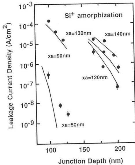
Fig.5 Variation of leakage current density for  $\text{Si}^+$  pre-amorphized samples. Solid lines indicate  $J^{\text{model}} = C/m \int N_{\text{int}}(x) dx$  for  $C/m = 2 \times 10^{-19}$ .
