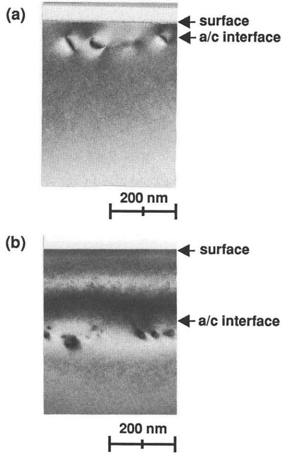
**Fig.4** Cross-sectional TEM images for  $\text{Si}^+(x_a=50\text{nm})$  (a) and  $\text{Ge}^+(x_a=220\text{nm})$  (b) samples after 1000°C/15sec annealing.
