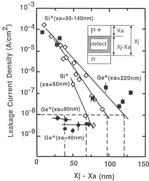
**Fig.3** The dependence of leakage current density on the  $x_j-x_a$  for several pre-amorphized layer thickness  $x_a$  formed by  $\text{Si}^+$  and  $\text{Ge}^+$  implantations. For  $\text{Si}^+$  pre-amorphized samples,  $x_a=50\text{nm}$  ( open circles),  $x_a$  is in the range from 90 to 140nm ( open diamonds ). For  $\text{Ge}^+$  pre-amorphized samples,  $x_a=40\text{nm}$  ( closed circles ),  $x_a=90\text{nm}$  ( closed diamonds ) and 220nm ( closed squares ).
