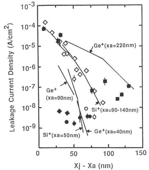
Fig.6 The dependence of leakage current density on the  $x_j - x_a$  for several pre-amorphized layer thickness  $x_a$  formed by  $\text{Si}^+$  and  $\text{Ge}^+$  implantations. Solid lines indicate  $J^{\text{model}} = C/m \int N_{\text{int}}(x) dx$  for  $C/m = 2 \times 10^{-19}$ .
