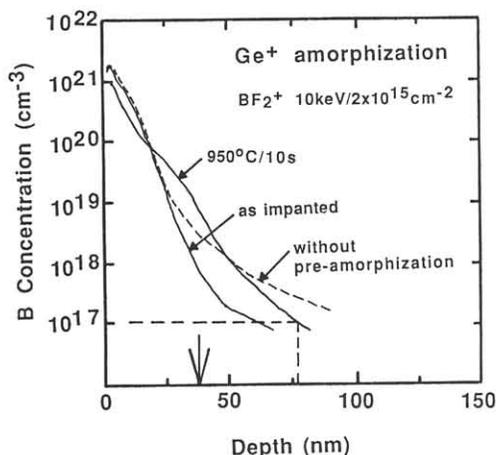
Fig.1 B profiles for pre-amorphized and crystal samples. The arrow indicates the a/c interface position.
