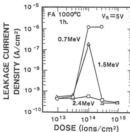
Fig. 1 Dose dependence of the junction leakage current at  $V_R=5V$  of diodes formed with a boron implanted buried layer at 0.7, 1.5 and 2.4 MeV.
