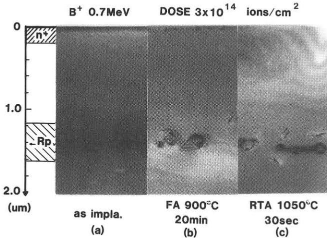
Fig. 6 Cross-sectional TEM photographs of the samples implanted at 0.7 MeV with a dose of  $3 \times 10^{14}$  ions/cm<sup>2</sup>. (a) As implanted, (b) FA at 900°C for 20 mins and (c) RTA at 1050°C for 30 secs.
