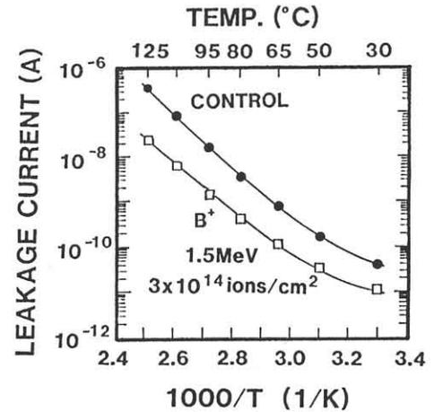
Fig. 9 Temperature dependence of the junction leakage current of diodes with and without a p<sup>+</sup> buried layer.
