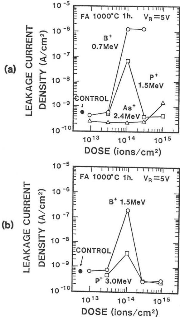
Fig. 7 Dose dependence of the junction leakage current of diodes with a buried layer, (a)  $R_p=1.4\mu\text{m}$ ; i.e. 0.7 MeV boron, 1.5 MeV phosphorus and 2.4 MeV arsenic (b)  $R_p=2.4\mu\text{m}$ ; i.e. 1.5 MeV boron and 3.0 MeV phosphorus.
