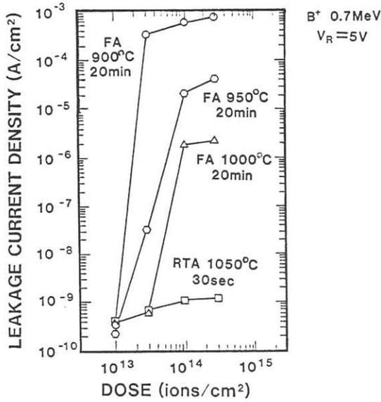
Fig. 5 Dose dependence of the junction leakage current at  $V_R=5V$  of diodes implanted with 0.7 MeV boron and annealed at 900°C, 950°C and 1000°C for 20 mins (FA) and at 1050°C for 30 secs (RTA).
