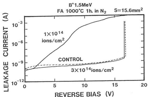
Fig. 2 Reverse bias I-V characteristics of n<sup>+</sup>/p diodes with a boron implanted buried layer at 1.5 MeV
