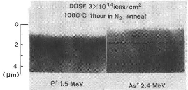
Fig. 8 Cross-sectional TEM photographs of the samples implanted with 1.5 MeV phosphorus and 2.4 MeV arsenic.
