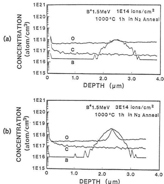
Fig. 4 SIMS depth profiles of boron, carbon and oxygen measured on samples implanted with (a)  $1 \times 10^{14}$  and (b)  $3 \times 10^{14}$  ions/cm<sup>2</sup> boron at 1.5 MeV and annealed at 1000 °C for 1 hour.
