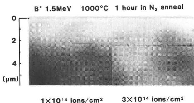
Fig. 3 Cross-sectional TEM photographs of secondary defects for boron implantation at 1.5 MeV with a dose of  $1 \times 10^{14}$  and  $3 \times 10^{14}$  ions/cm<sup>2</sup>, and annealed at 1000 °C for 1 hour.
