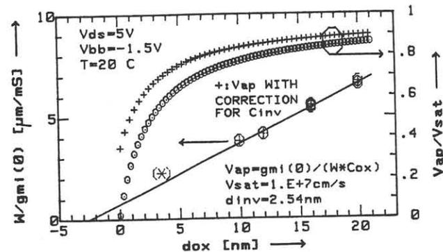
Figure 8. Maximum possible intrinsic transconductance of nMOSFETs determined by extrapolating to zero channel length vs oxide thickness. The apparent carrier velocities  $V_{ap}$  with and without correction for  $C_{inv}$  are shown, too.
