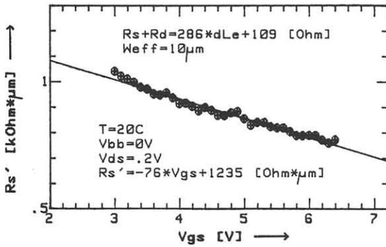
Figure 1. Gate voltage dependent source series resistance of nMOSFETs with LDD extensions  $R_s'$  normalized to  $1 \mu\text{m}$  channel length.
