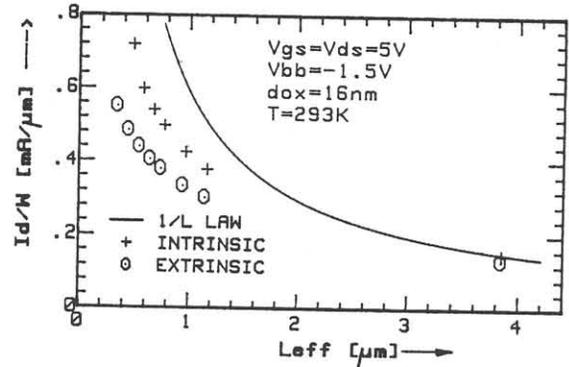
Figure 5. Channel length dependent drain current of the extrinsic, intrinsic and the ideal nMOSFETs determined by auto-correction for  $R_s$  and  $R_d$ .
