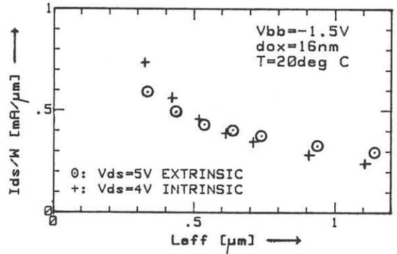
Figure 6. Comparison of the drain currents of the extrinsic nMOSFETs with 5V and the intrinsic nMOSFETs with 4V operation voltages.
