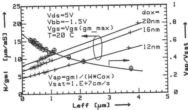
Figure 7. The intrinsic transconductance of nMOSFETs vs. effective channel length for different oxide thicknesses.
