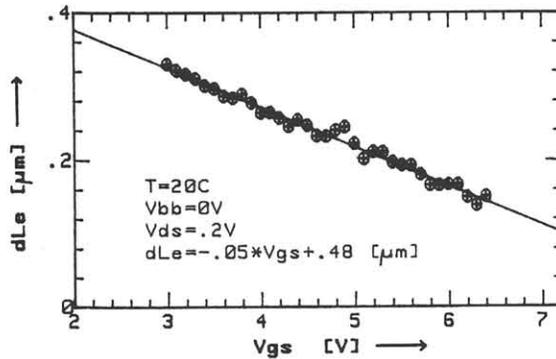
Figure 2. Gate voltage dependent effective channel length defined by  $dL_e = L_g - L_{eff}$  for nMOSFETs with LDD extensions.
