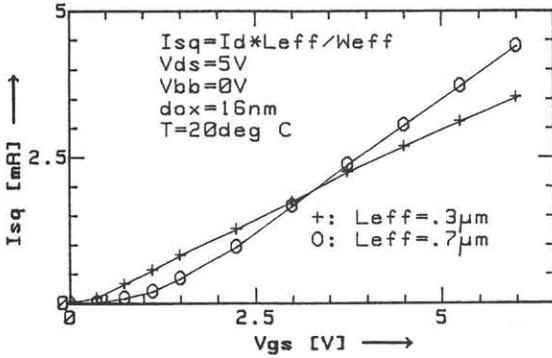
Figure 3. Drain current of square nMOSFETs  $I_{sq}$  for two different channel lengths as a function of the gate voltage  $V_{gs}$ .
