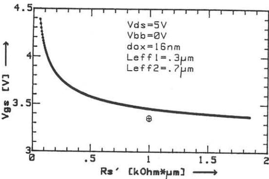
Figure 4. The cross-point gate voltage vs. source series resistance  $R_s'$  calculated for drain currents of square nMOSFETs with two different channel lengths.
