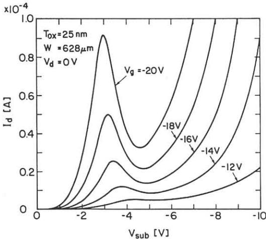
Fig.2 Typical  $I_d$ - $V_{sub}$  characteristics. The  $I_d$ - $V_{sub}$  curve for each  $V_g$  was measured by sweeping  $V_{sub}$  from 0 to -10 V and at fixed  $V_d = 0$  V.
