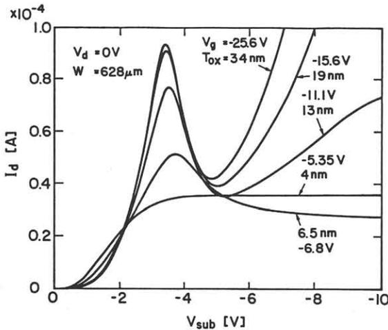
Fig.3  $I_d$ - $V_{sub}$  characteristics for various gate oxide thicknesses. Gate bias values are -25.6, -15.6, -11.1, -6.8, -5.35 V for  $T_{ox} = 34, 19, 13, 6.5, 4$  nm, respectively.
