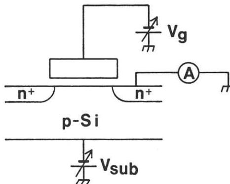
Fig.1 Schematic cross section of the MOSFET.
