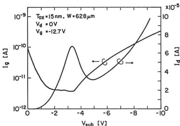
Fig.6  $I_g$ - $V_{sub}$  characteristic for  $T_{ox} = 15$  nm at  $V_g = -12.7$  V.
