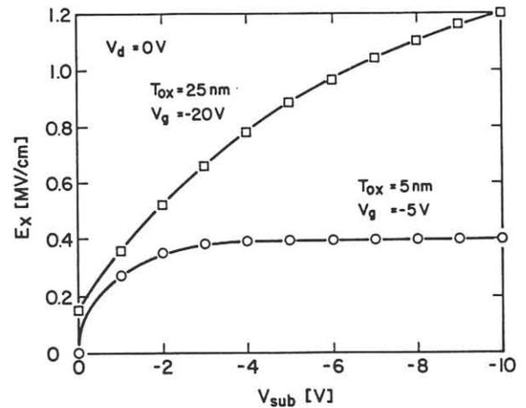
Fig.8 Calculated lateral electric field  $E_x$  for  $T_{ox} = 25$  and  $5$  nm by 2-dimensional device simulator.  $V_g = -20$  and  $-5$  V for  $T_{ox} = 25$  and  $5$  nm, respectively.
