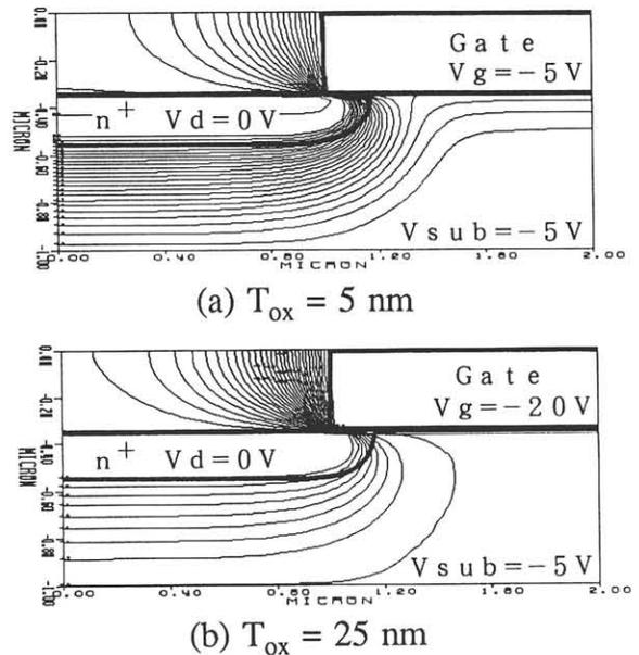
Fig.9 Potential distribution contour plot at  $V_{sub} = -5$  V. (a) When  $T_{ox} = 5$  nm. (b) When  $T_{ox} = 25$  nm.  $V_g$  values are  $-5$  and  $-20$  V for  $T_{ox} = 5$  and  $25$  nm, respectively.
