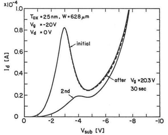
Fig.4  $I_d$ - $V_{sub}$  characteristic at initial and 2nd  $V_{sub}$  sweeping. The dashed line curve indicates I-V characteristics after being biased at  $V_g = 20.3$  V for 30 sec.
