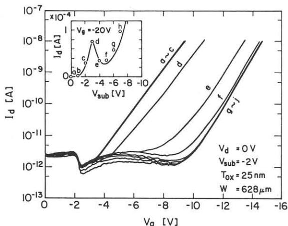
Fig.5  $I_d$ - $V_g$  characteristic for  $V_{sub} = -2$  V after 0.2 sec stressing at  $V_{sub}$  and  $V_g = -20$  V.
