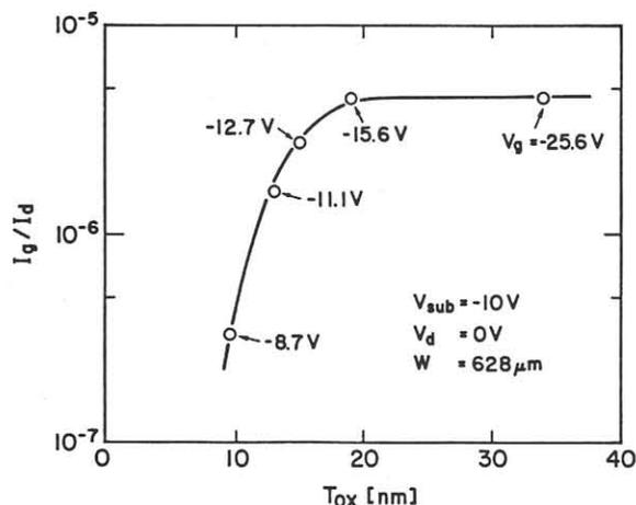
Fig.7  $T_{ox}$  dependence of the  $I_g/I_d$  ratio at  $V_{sub} = -10$  V. The gate bias values are -25.6, -15.6, -12.7, -11.1, -8.7 V for  $T_{ox} = 34, 19, 15, 13, 9.5$ , respectively.
