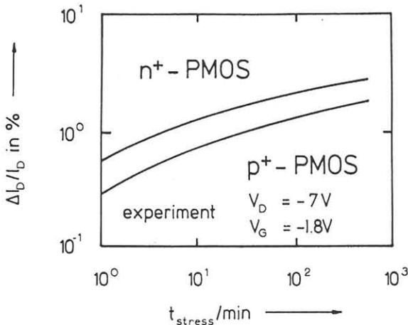
Fig. 4 Time evolution of drain current during stress: experimental data.
