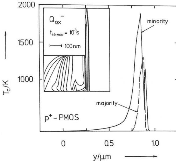
Fig.7 Minority and majority carrier temperatures along the interface for p<sup>+</sup> PMOS. The insert shows the trap distribution at  $t=10^3$  sec.
