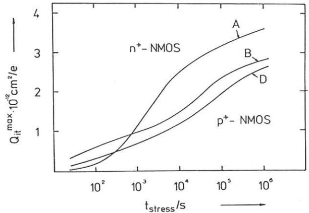
Fig.2 Time evolution of maximum interface state charge during stress experiment. A and B are the devices specified in Fig.1. The device D is a buried channel device with  $1.8 \times 10^{12} cm^{-2}$ , 160keV As compensation implant.
