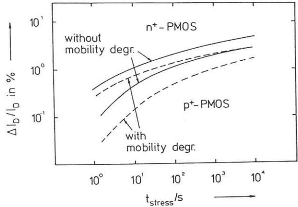
Fig. 5 Time evolution of drain current during hot-carrier stress: simulated data. Solid lines - no mobility degradation, dashed lines - maximum mobility degradation.
