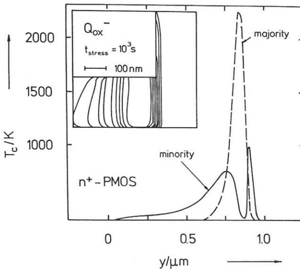
Fig.8 Minority and majority carrier temperatures along the interface for n<sup>+</sup> PMOS. The insert shows the trap distribution at  $10^3$  sec.
