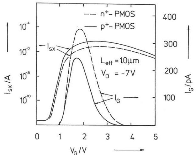
Fig. 6 Substrate and gate currents for n<sup>+</sup> and p<sup>+</sup> gate PMOS: experimental data.
