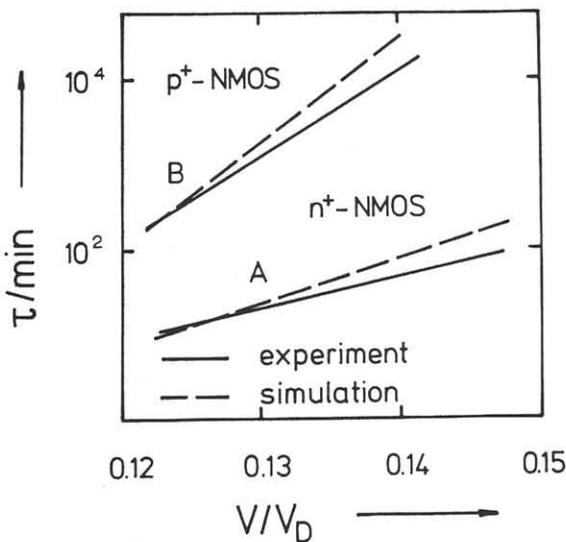
Fig.1 Comparison of life time of p<sup>+</sup> and n<sup>+</sup> NMOS devices with effective channel length  $L_{eff}=0.8\mu m$ . Solid line - experiment, dashed line - simulation. A is a surface channel LDD and B a buried channel device with As compensation doping of  $1.4 \times 10^{12} cm^{-2}$ , 100keV and identical S/D complex as A.
