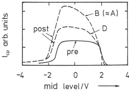
Fig. 3 Charge-pumping current prior and after stress for devices specified in Fig.'s 1 and 2.
