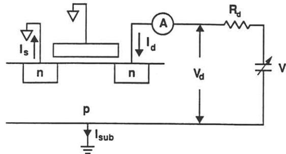
Fig. 1 Experimental set up for BV<sub>dss</sub> measurement, normally  $R_d=0$ .
