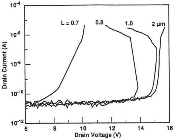
Fig. 3 I-V breakdown/snapback curve for  $L = 0.7, 0.8, 1.0$  and  $2.0 \text{ }\mu\text{m}$ .
