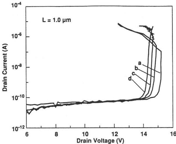
Fig. 4 I-V breakdown curve for different gate biases, (a)  $V_g = 0$ , (b)  $V_g = -0.5 \text{ V}$ , (c)  $V_g = -1.0 \text{ V}$ , (d)  $V_g = -1.5 \text{ V}$
