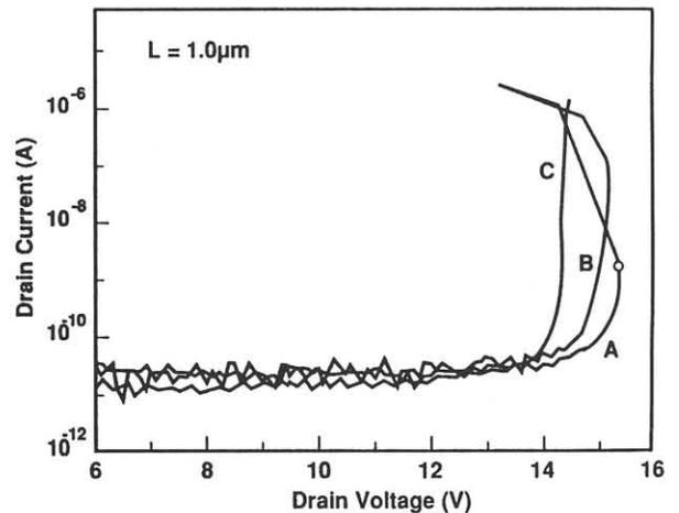
Fig. 7 I-V snapback curve for three different p well doses, A:  $1.4 \text{ E}12/\text{cm}^2$ , B:  $2.5 \text{ E}12/\text{cm}^2$ , C:  $1.0 \text{ E}13/\text{cm}^2$
