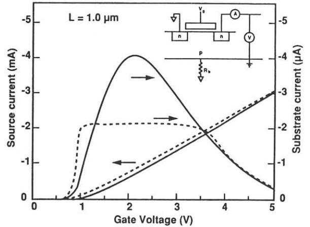
Fig. 5 Source and substrate current with (dashed) and without (solid) external substrate resistor  $R_b = 300 \text{ k}\Omega$  as shown in the insert.
