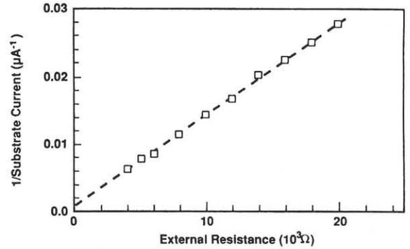
Fig. 6  $1/I_{\text{sub}}$  versus external substrate resistance
