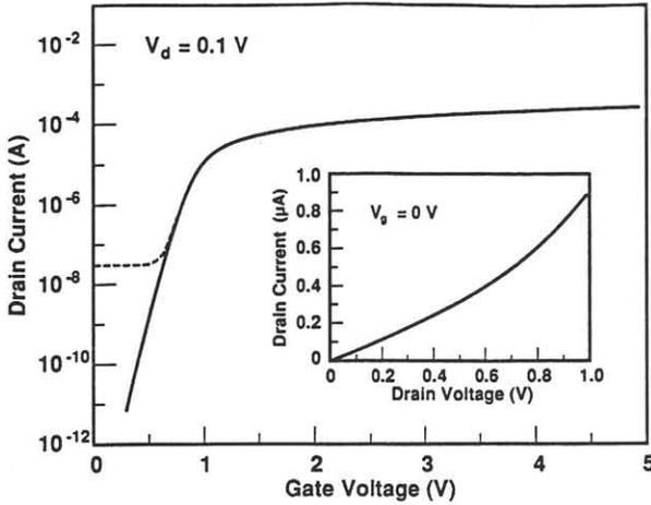
Fig. 2 Transistor transfer curve measured before (solid) and after (dashed) BVDss measurement. The leakage current after is a resistive short between source and drain as shown in the inset.
