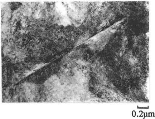
Fig.2 TEM image for films crystallized after phosphorus implantation. (15keV and  $1 \times 10^{13} \text{ cm}^{-2}$ ) (600°C and 40hours)
