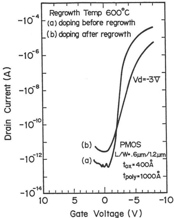
Fig.7 TFT characteristics.
