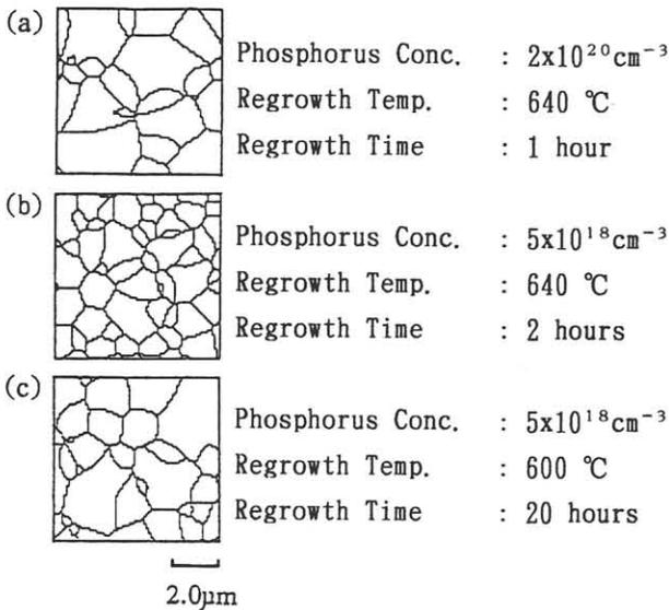
Fig.5 Feature of grains simulated under various conditions.
