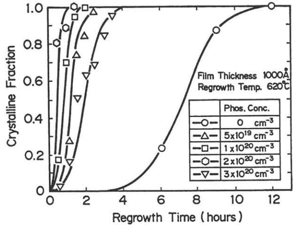
Fig.3 Crystalline fraction vs. annealing time.
