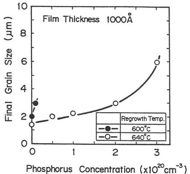
Fig.6 Grain size dependence on phosphorus concentration.
