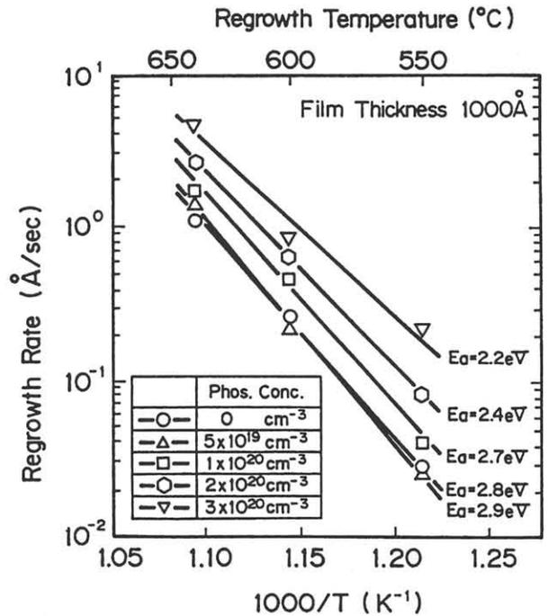
Fig.4 Regrowth rate vs. annealing temperature. Activation energies are also shown.
