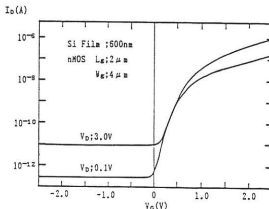
Fig.5 Subthreshold characteristics of the fabricated nMOS. A subthreshold swing of  $104\text{mV}/\text{decade}$  is obtained.
