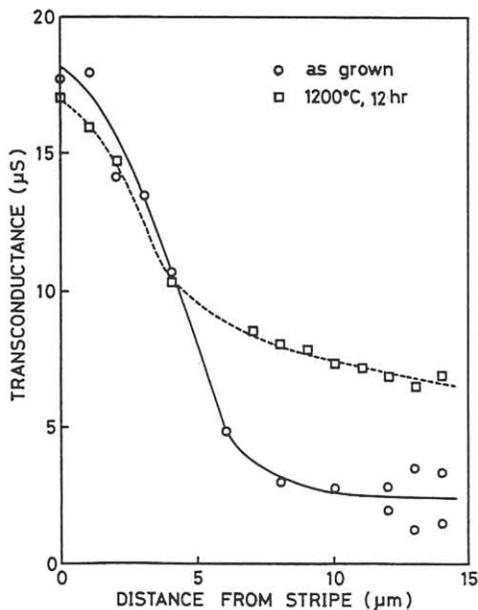
Fig.6 Transconductance of the fabricated MOSFETs as a function of the distance from the stripe edge.
