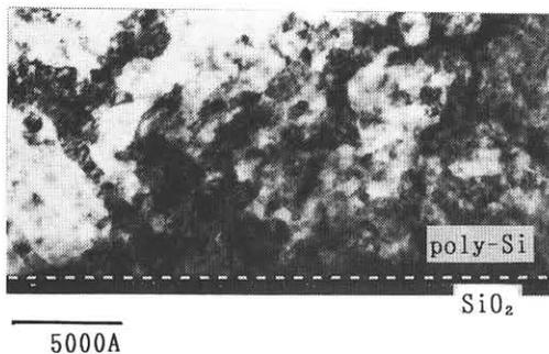
Fig.3 Cross sectional transmission electron micrograph of the avalanche nucleated layer.
