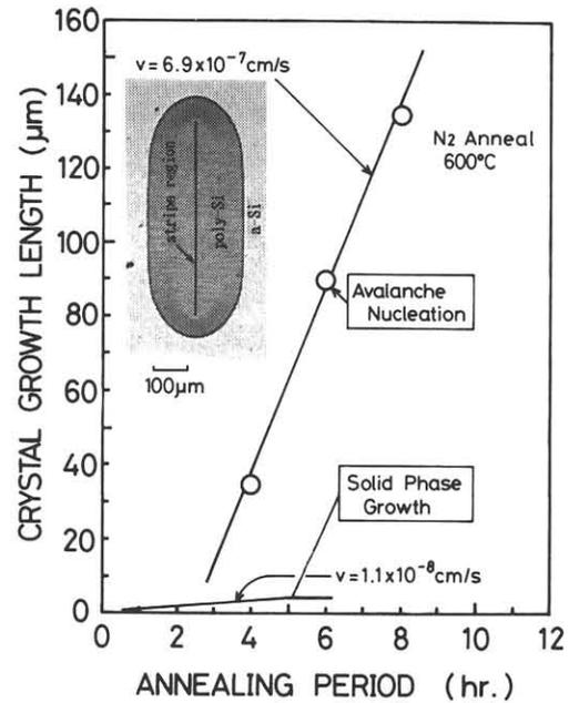
Fig.1 Crystal growth characteristics of avalanche nucleation. Inset shows optical micrograph of the sample after Wright etching.
