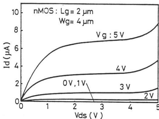
Fig.4  $I_d$ - $V_d$  characteristics of the fabricated nMOS.
