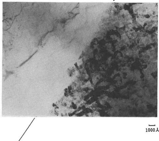
Fig.2 Transmission electron micrograph of the avalanche nucleated layer in the vicinity of the stripe region.
