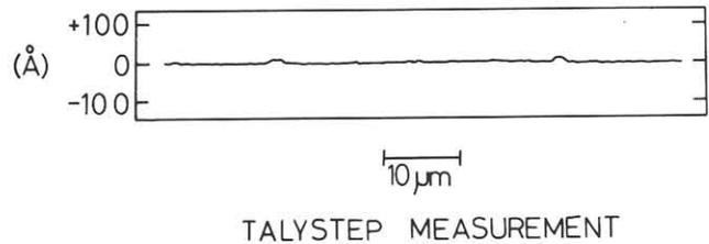
Fig.5 Talystep profile of a 60nm-thick- $\text{In}_{0.15}\text{Ga}_{0.85}\text{As}$  layer grown on GaAs.
