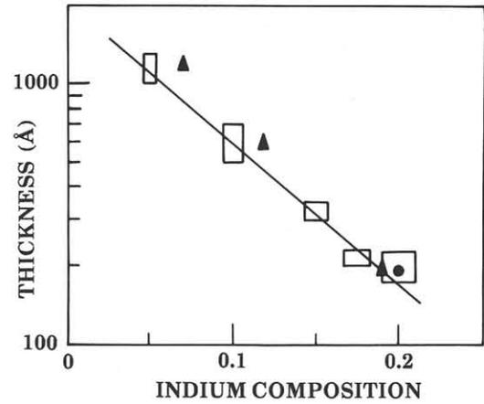
Fig.4 Critical layer thickness for the onset of roughness vs the indium composition. The results are plotted as error areas. The critical layer thickness for the generation of dislocations determined by Gourley et al<sup>1</sup>) (●) and Morris et al<sup>2</sup>) (▲) is also shown.
