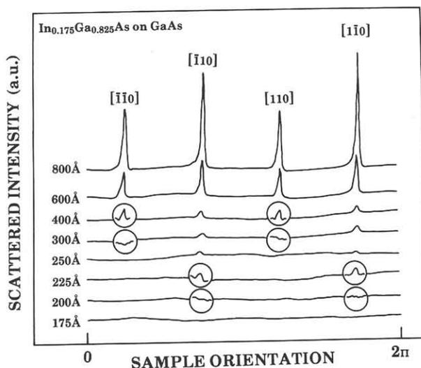
Fig.3 Azimuthal spectra of the scattered light intensity obtained during the growth of  $\text{In}_{0.175}\text{Ga}_{0.825}\text{As}$  on GaAs. The total InGaAs layer thickness is indicated for each spectrum. The intensity is magnified by a factor of 5 in the encircled insets.
