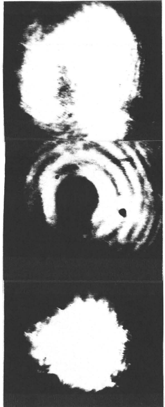
Fig.6 Far field beam patterns of (a) a 2 x 3 periodic array, (b) a hexagonal array and (c) a centered hexagonal array.
