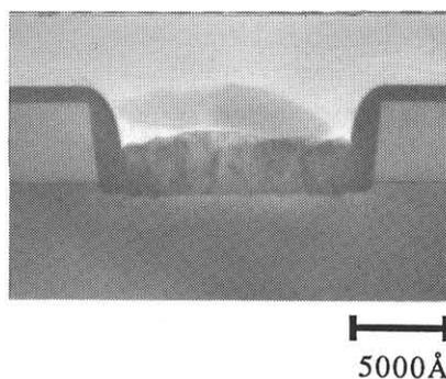
Fig. 6 Cross-sectional TEM image of the 3000Å thick SPD film on a Si<sub>3</sub>N<sub>4</sub> window.
