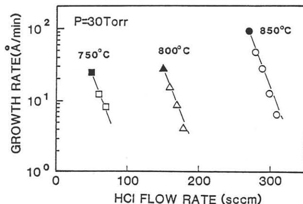
Fig. 3 Growth rate as a function of HCl flow rate for different temperatures.
