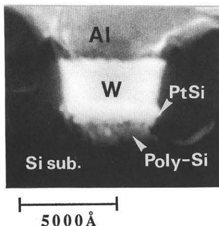
Fig. 8 Cross-sectional SEM image of the buried emitter electrode structure.
