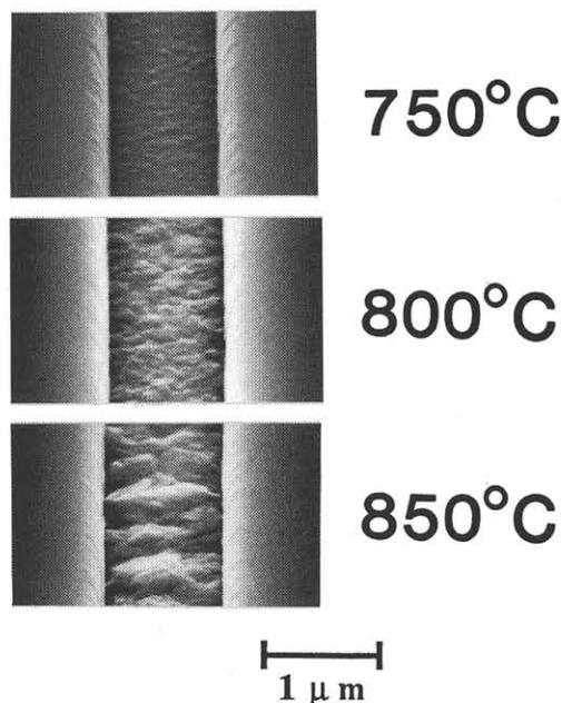
Fig. 5 SEM images of the polysilicon film deposited at 30 torr.
