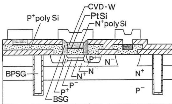
Fig. 2 Schematic cross-section of the Advanced BSA transistor.
