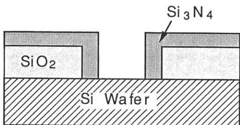
Fig. 1 Schematic cross-section of the  $\text{Si}_3\text{N}_4$  window.
