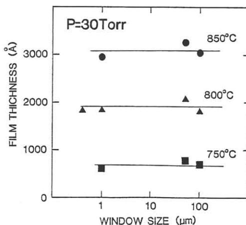
Fig. 7 SPD film thickness as a function of window size.
