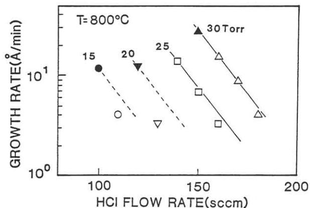
Fig. 4 Growth rate as a function of HCl flow rate for different pressures.
