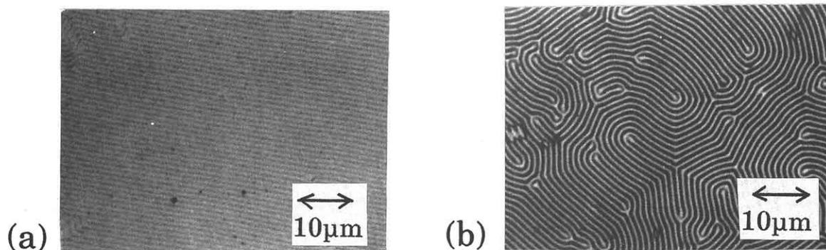
Fig.1 Photomicrographs of magnetic domains measured by Bitter method: (a) a magnetic domain for (110)  $(\text{BiY})_3\text{Fe}_5\text{O}_{12}$  and (b) a conventional magnetic domain for (111).
