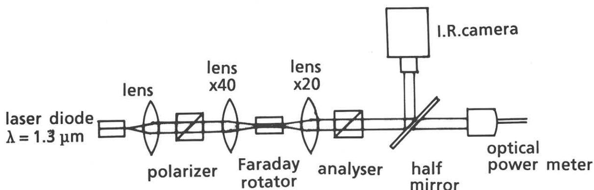
Fig.3 experimental setup to measure the Faraday rotation angle and the extinction ratio.
