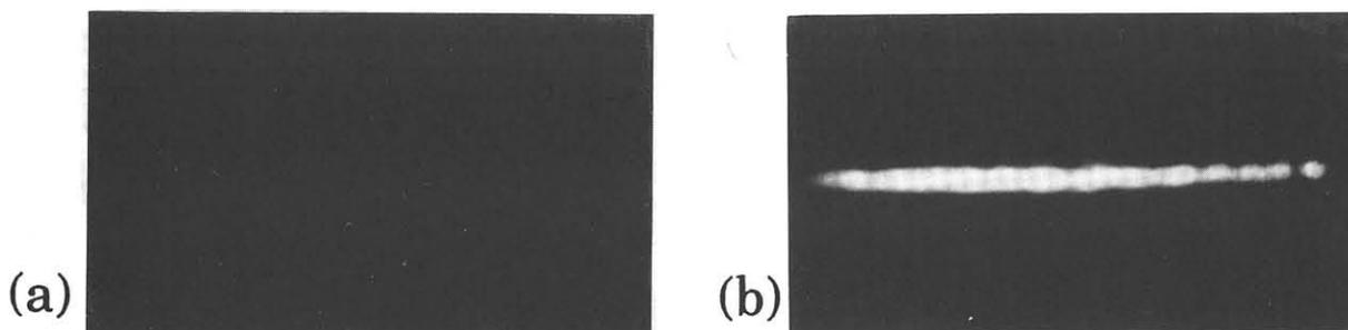
Fig.4 Photographs of the guided lightwave in the Faraday rotator: (a) with the analyzer set at the extinction angle and (b) at the angle of  $+90$  deg.
