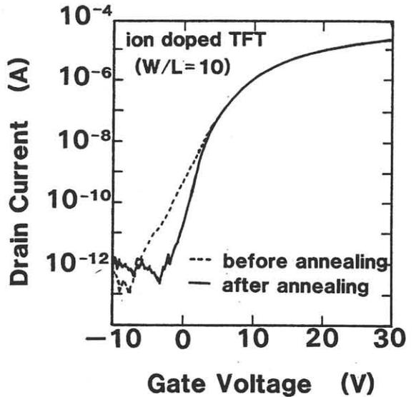
Figure 5  $V_G$ - $I_D$  characteristic of fabricated TFT ( $V_D=12V$ ,  $L=10\mu m$ ,  $W=100\mu m$ ).  $V_{TH}$  is 4.8V and field effect mobility is  $0.58 \text{ cm}^2/Vs$ .
