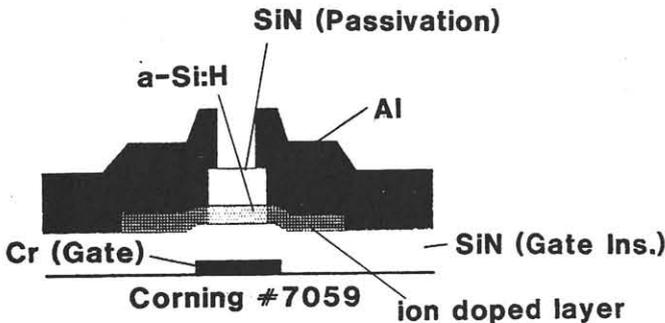
Figure 4 Cross-sectional view of fabricated TFT
