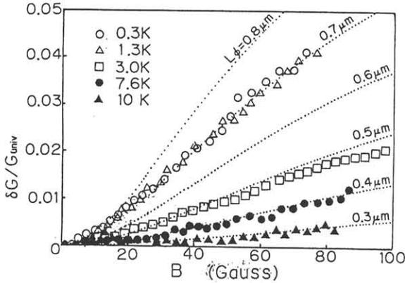
Fig. 1 Magnetoconductance spectra of a gated AlGaAs/GaAs quantum wire (#12) measured at temperatures varying from 0.3K to 10K. The dotted lines show the theoretical fittings of the BvH theory.
