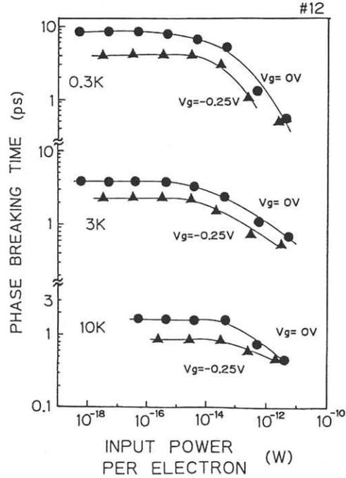
Fig. 3 Phase breaking time  $\tau_{\phi}$  as functions of input power per electron at various lattice temperatures.
