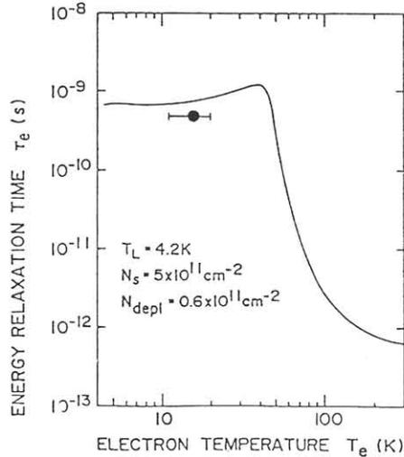
Fig. 4 Calculated energy relaxation time for two-dimensional electrons in a selectively doped AlGaAs/GaAs heterojunction by assuming phonon scatterings. The parameters used in the calculation are shown in the figure. The circle shows the measured energy relaxation time in the AlGaAs/GaAs quantum wire.
