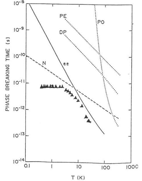
Fig. 2 Temperature dependence of the phase breaking time  $\tau_\phi$ . Calculated phase breaking times limited by electron-electron scattering and by phonon scatterings are also shown; DP: deformation potential scattering, PE: piezoelectric scattering, PO: polar optical phonon scattering, ee: momentum-conserving electron-electron scattering, N: scattering by electromagnetic fluctuation.
