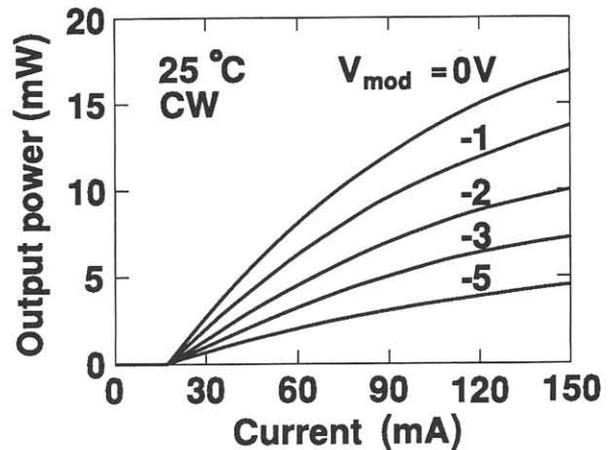
Fig.2 Light output versus current characteristics.
