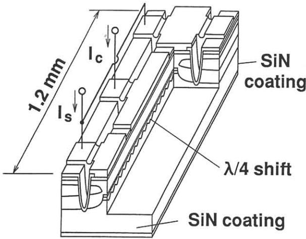
Fig.4 Schematic structure of 3-electrode long cavity  $\lambda/4$  shifted DFB laser.
