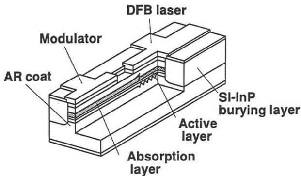
Fig.1 Schematic structure of electro-absorption/DFB laser light source.
