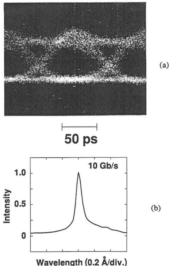
Fig.3 Eye pattern and the spectrum under 10 Gb/s NRZ modulation.
