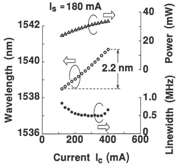
Fig.5 Wavelength, linewidth and output power characteristics.
