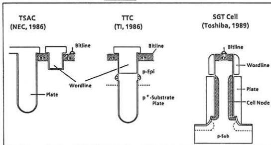
Fig. 4 Trench transistor cell concepts
