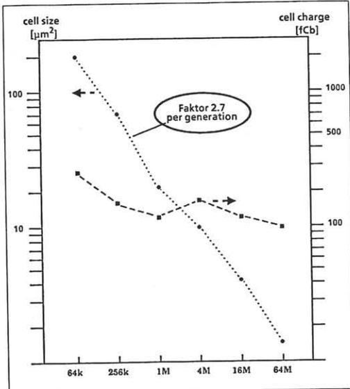
Fig. 2 Evolution of one transistor cell size and of cell charge. A cell capacitance of 30 fF is assumed for 64M
