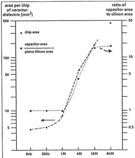
Fig. 5 Increase of area of varactor dielectric per chip and area ratio ("folding efficiency") from 64k to 64M.
