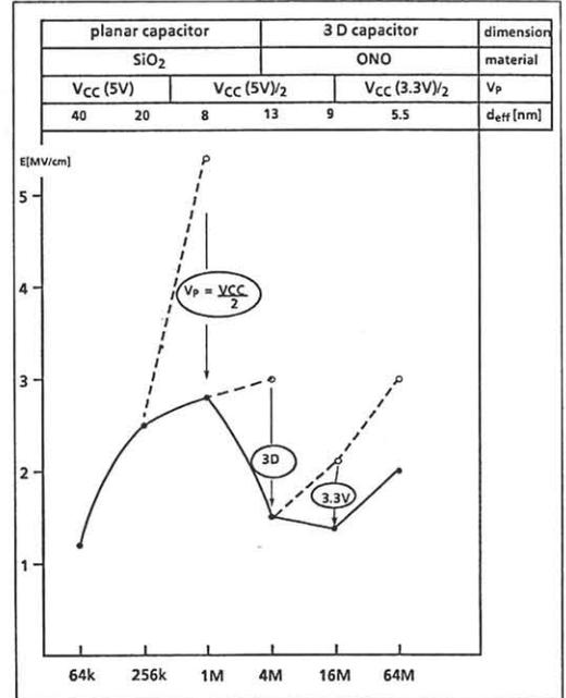
Fig. 6 Electric field exerted on capacitor dielectric. The measures to keep the field well below 3 MV/cm are indicated.
