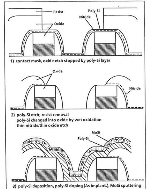
Fig. 7 Process flow for selfaligned bitline contact formation using an oxidizable etchstop layer<sup>5)</sup>
