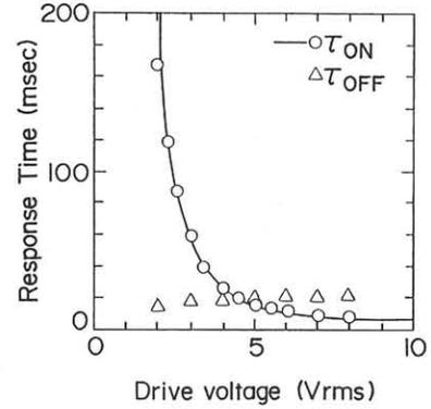
Fig.3 Response time of the transmission as a function of drive voltage of the TN-LC cell:  $\circ$  is measured  $\tau_{ON}$ ,  $\Delta$  is measured  $\tau_{OFF}$ , solid line is calculated  $\tau_{ON}$  using eq.(7).
