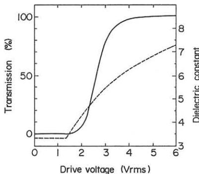
Fig.2 Transmission-Voltage characteristics (solid line) and Dielectric Constant-Voltage characteristics (dashed line) of the TN-LC cell.
