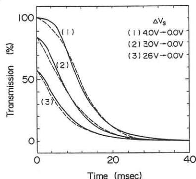
Fig.5 Measured(solid line) and calculated (dashed line) optical fall characteristics of the TN-LC cell.
