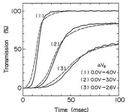
Fig.4 Measured(solid line) and calculated (dashed line) optical rise characteristics of the TN-LC cell.
