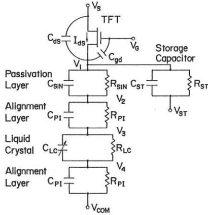
Fig.1 A pixel equivalent circuit.
